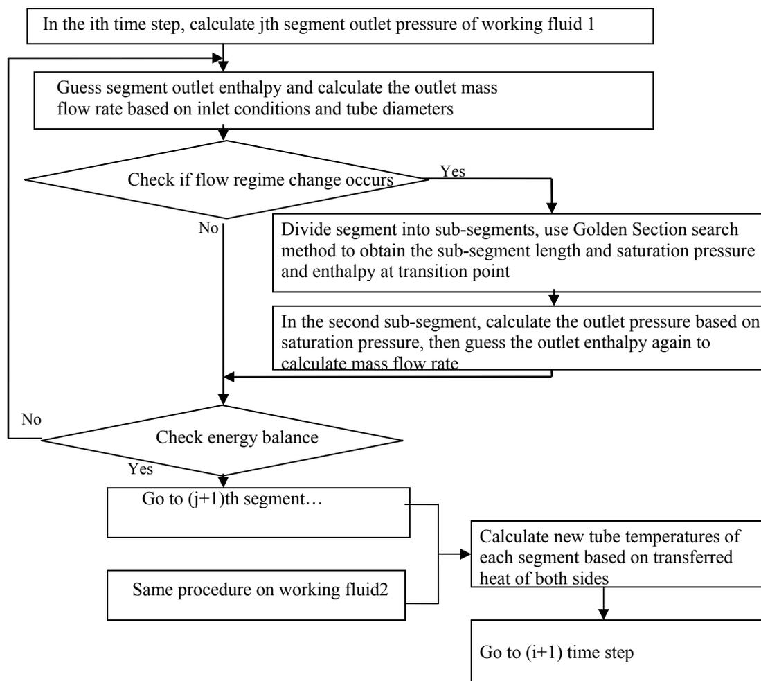
Figure 1: Flow chart of the algorithm
