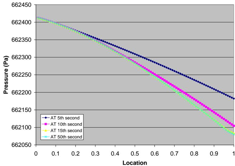
Figure 3: Pressure Distribution of an Air to Refrigerant Heat Exchanger
