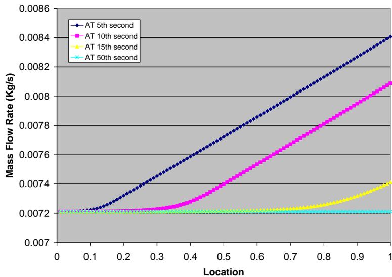
Figure 4: Mass Flow Rate Profile in an Air to Refrigerant Heat Exchanger
