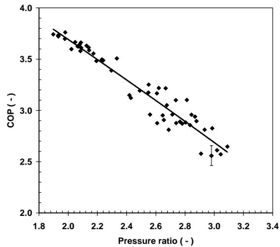
Figure 7: Coefficient of performance versus refrigerant pressure ratio.
