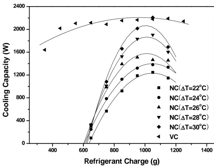
Figure 4 : Effect of the refrigerant charge with receiver.
