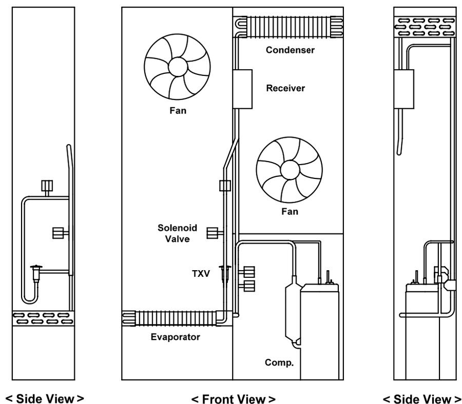
Figure 2 : Layout of the tested cooler.
