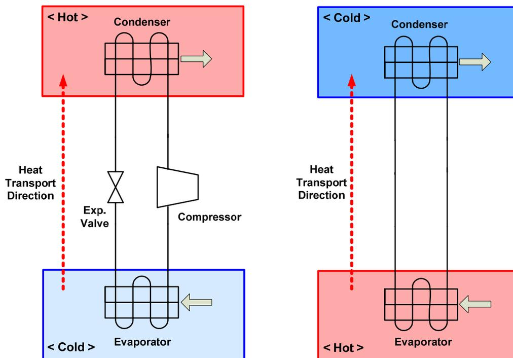
Figure 1 : Schematic of hybrid cooler.
