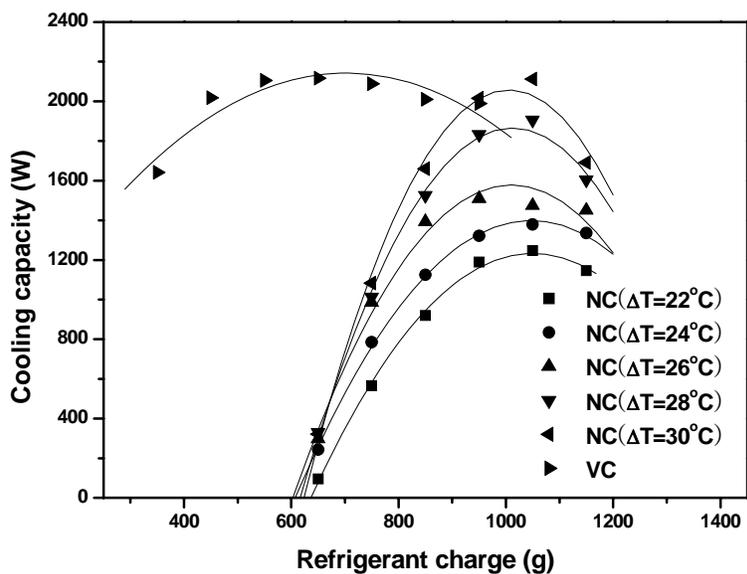
Figure 3 : Effect of the refrigerant charge without receiver.
