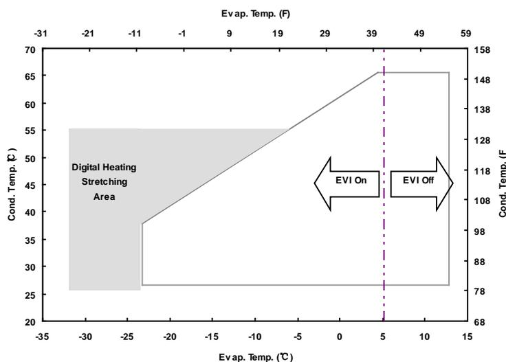
Figure 3: the Digital Heating Scroll Compressor Envelop
