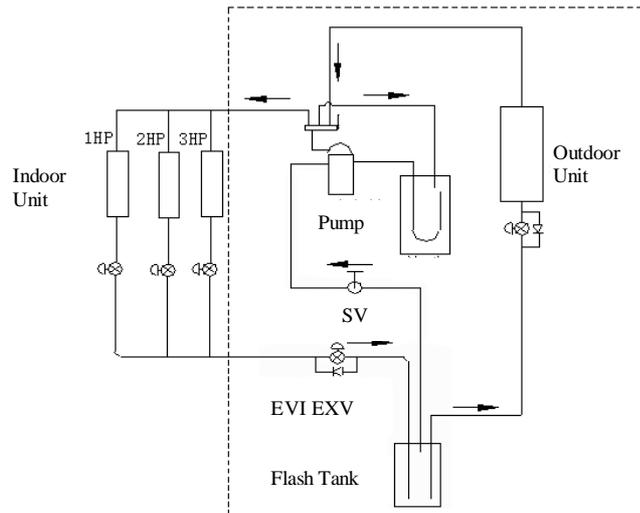
Figure 5: Central AC Heat Pump System Layout
