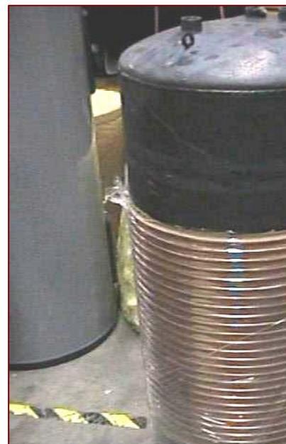
Figure 1: Cutaway schematic view of existing integral HPWH product (left side) and photo of tank with condenser installed (right side)
