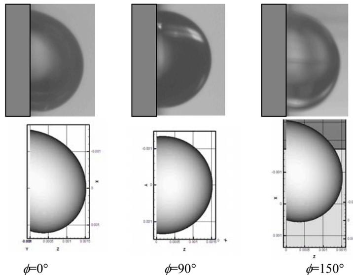
Figure 4: A comparison of the shape of a drop on surface A captured using a digital camera from three different azimuthal angles ( $\phi$ , the picture shows a side view to the drop/bridge when  $\phi=0^\circ$ ), to the predicted shape.
