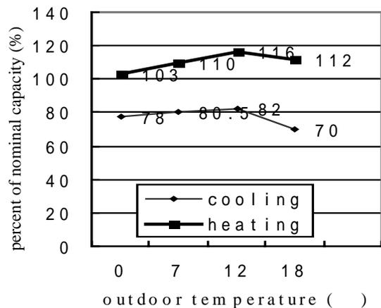
Figure 7: Curves of the percent of nominal capacity in the heating-principal mode at combination 3
