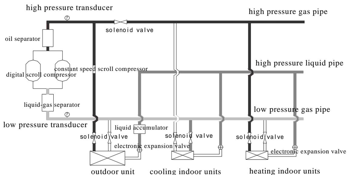
Figure 1: Schematic diagram for the new type three pipes heat recovery GMV-R300W2/Rh unit
