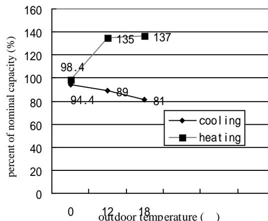
Figure 8: Curves of the percent of nominal capacity in the heating-principal mode at combination 4
