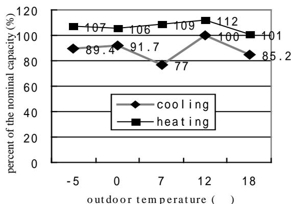
Figure 5: Curves of the percent of nominal capacity in the cooling-principal mode at combination 1
