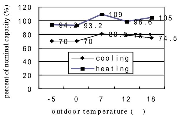
Figure 6: Curves of the percent of nominal capacity in the cooling-principal mode at combination 2
