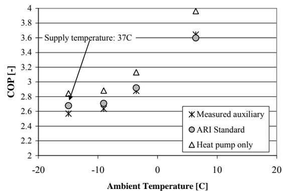
Figure 7: Coefficient of Performance considering the auxiliary power according to ARI guidelines and according to the measured values
