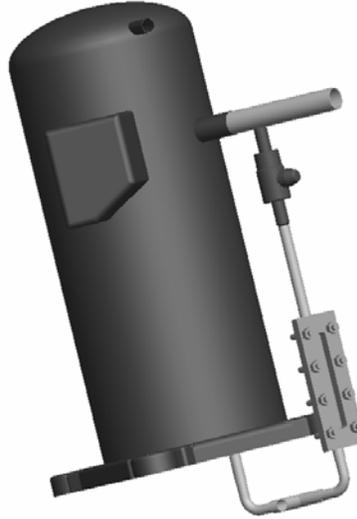
Figure 5: Schematic of the compressor with the sight glass for the determination of the oil level
