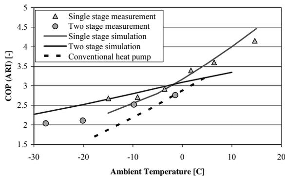
Figure 11: COP considering auxiliary power for the measurement, simulation and a conventional heat pump
