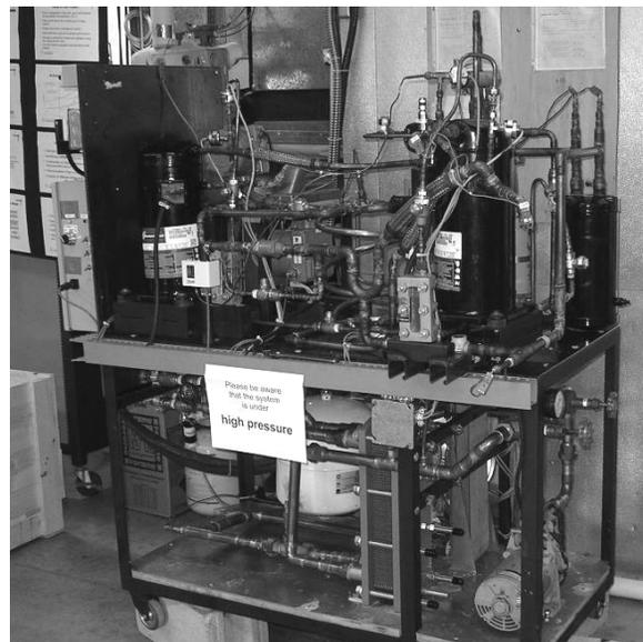
Figure 3: Picture of the main unit of the two stage heat pump cycle
