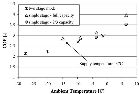
Figure 6: Coefficient of Performance not considering any auxiliary power consumption
