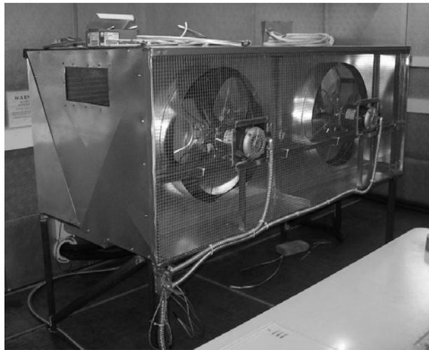
Figure 4: Picture of the outdoor heat exchanger with the angled coil located at the back and the two fans in front
