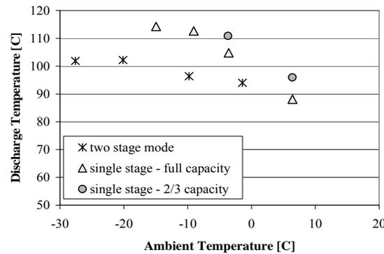
Figure 10: Discharge temperature of the high stage compressor in different operating modes
