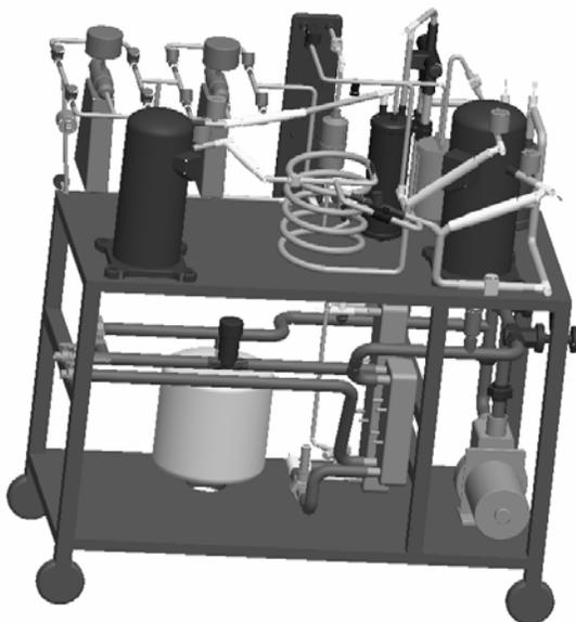
Figure 2: 3D - Design of the two stage heat pump cycle
