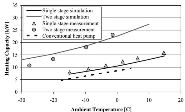
Figure 12: Heating capacity for the measurement, simulation and a conventional heat pump
