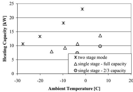
Figure 8: Heating capacity in different operating modes
