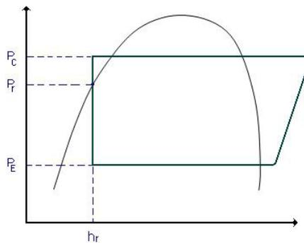
Figure 1: Schematic of the throttling process
