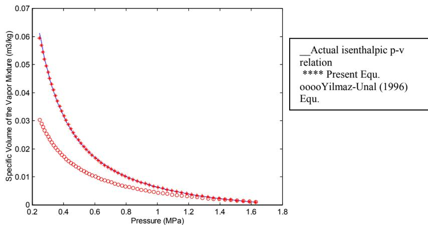
Figure 6: R407C  $P - v$  Relation for isenthalpic process for  $Pr = 17.37\text{ bar}$
