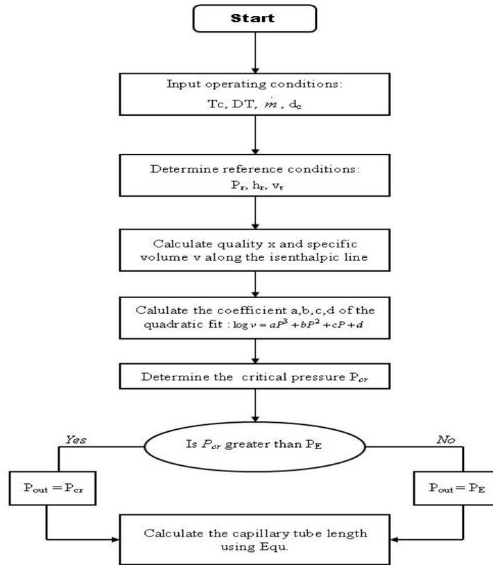
Figure 8: Flow chart for sizing capillary Tube
