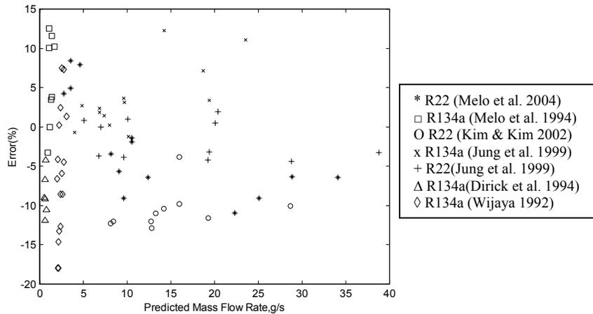
Figure 9: Comparison of predicted mass flow rates with data measured by other researchers.
