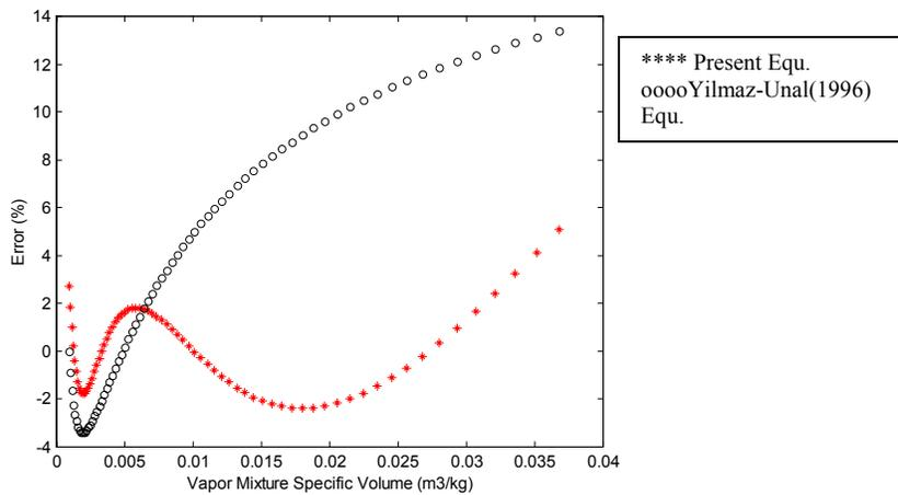
Figure 4: Deviation of specific volume for R22 at  $Pr = 19.427$  bar
