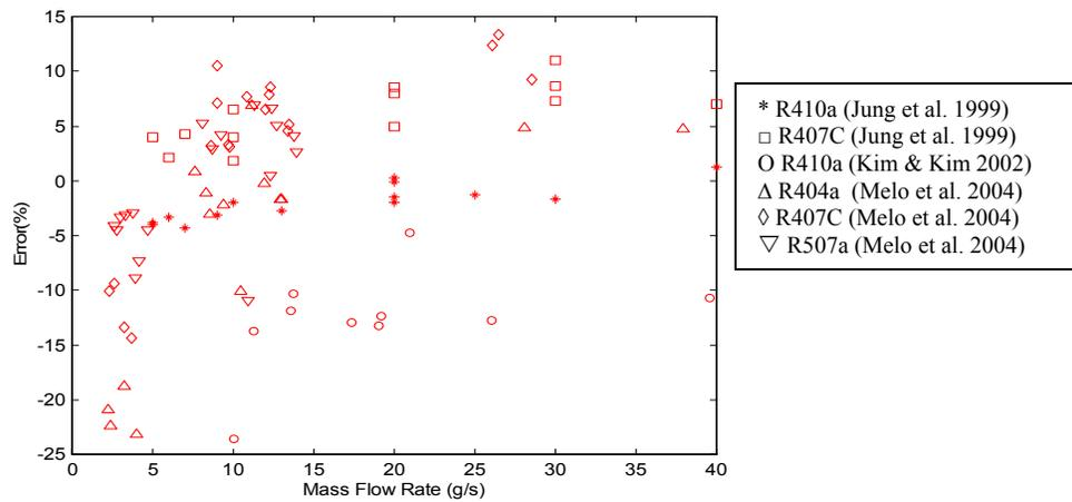
Figure 10: Comparison of predicted mass flow rates with data measured by other researchers.
