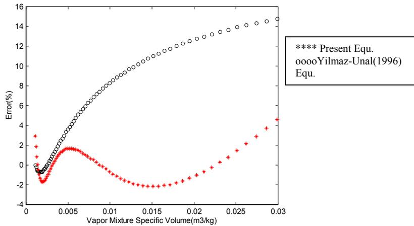
Figure 5: Deviation of specific volume for R410a at  $Pr = 30.65\text{bar}$
