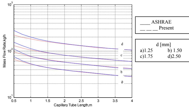
Figure 11: Variation of refrigerant mass flow rate with capillary tube length for R22 ( $P_C = 18 \text{ bar}$  and  $\Delta T_{sub} = 5.0^\circ C$ )
