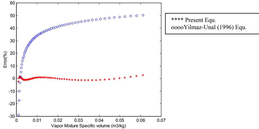
Figure 7: Deviation of specific volume for R407C at  $Pr = 17.37\text{bar}$
