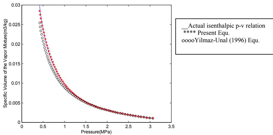
Figure 3: R410a  $P - v$  Relation for isenthalpic process for  $Pr = 30.65$  bar
