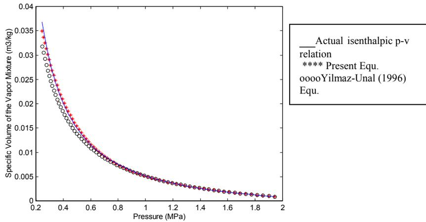
Figure 2: R22  $P - v$  Relation for isenthalpic process for  $Pr=19.427$  bar
