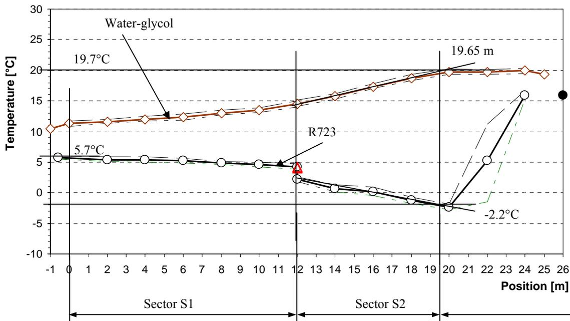
Figure 4: temperature profiles along the evaporator coils during test runs with evaporator *Sections 1* and *2* operated in series (Evaporation from  $x_{evap\_in} = 0.10$  to dry-out in Sectors S1 and S2, Superheating in Sector S3)
