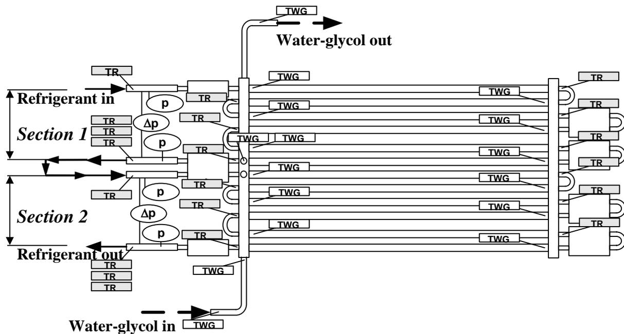
Figure 1: schematic arrangement of the measurement points on the evaporator
