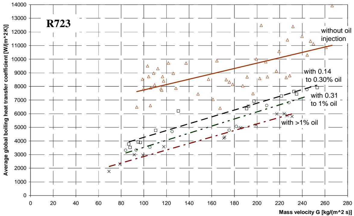
Figure 5: average global values of the boiling heat transfer coefficient  $h_{R723}$  for flow boiling of R723 versus mass flux for different oil contents.
