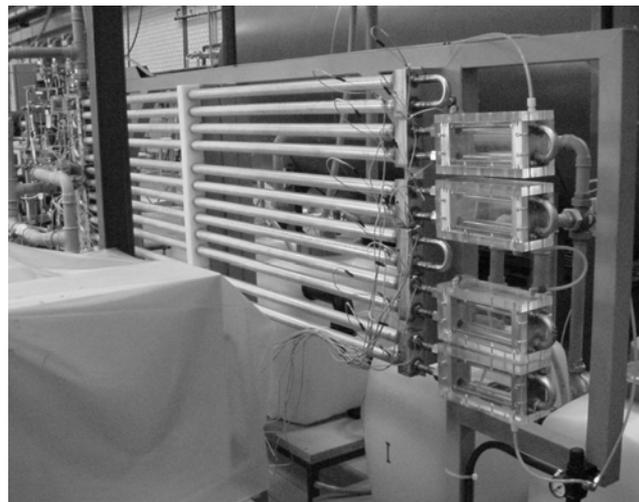
Figure 2: evaporator with sight glasses for observation of the flow regime
