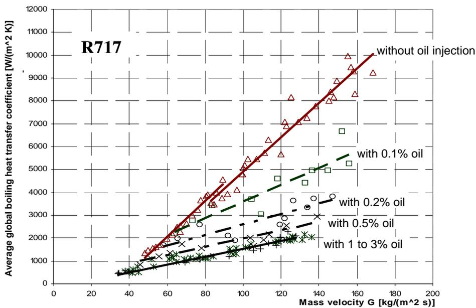
Figure 6: average global values of the boiling heat transfer coefficient  $h_{NH3}$  for flow boiling of ammonia (R717) versus mass flux for different oil contents.
