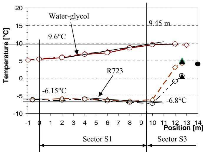
Figure 3: temperature profiles along the evaporator coils during test runs with evaporator *Sections 1* and *2* operated in parallel (Evaporation from  $x_{evap\_in} = 0.10$  to dry-out in Sector S1, Superheating in Sector S3)
