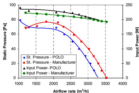
Figure 12: Static pressure and input power vs. airflow rate (350mm fan)
