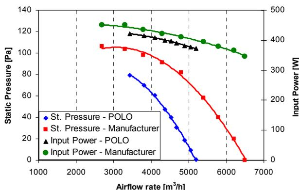
Figure 11: Static pressure and input power vs. airflow rate (450mm fan)
