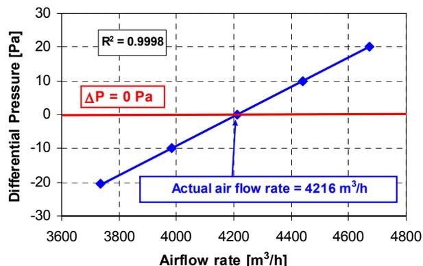
Figure 24: Operation point (3.5HP unit)
