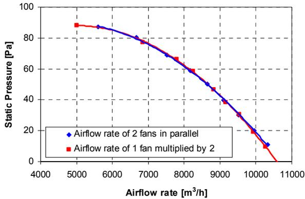
Figure 15: Static pressure versus airflow rate (450mm fan)
