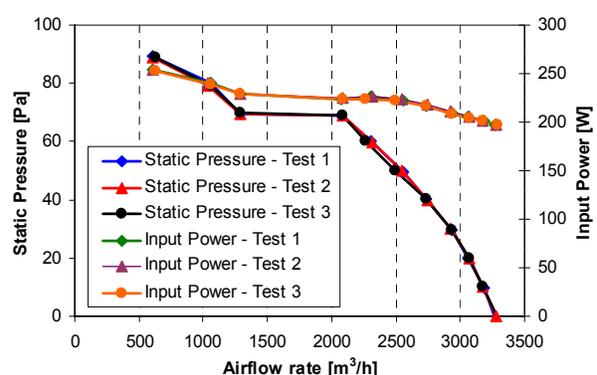
Figure 6: Static pressure and input power vs. airflow rate (350mm fan)
