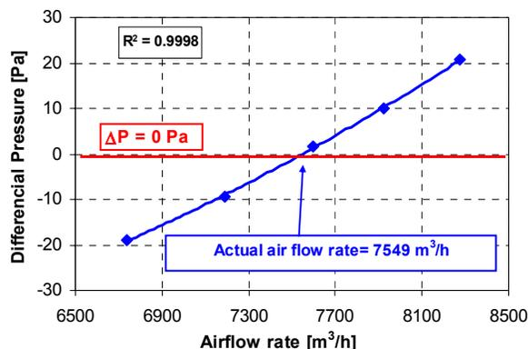
Figure 23: Operation point (5.0HP unit)
