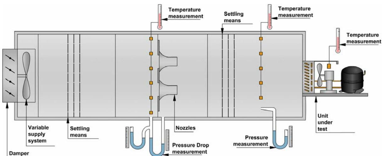
Figure 1: Diagram of the test apparatus
