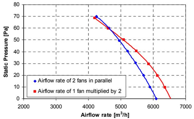
Figure 16: Static pressure versus airflow rate (350mm fan)
