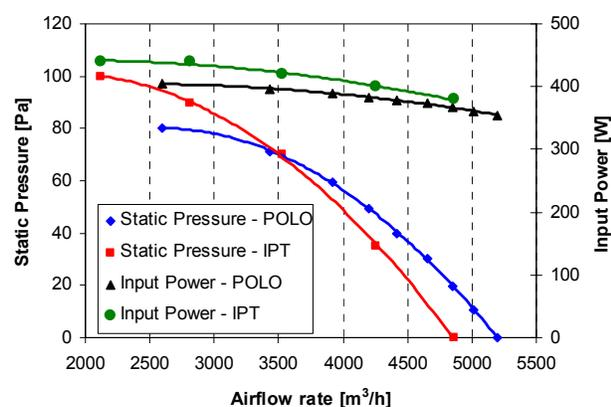
Figure 10: Static pressure and input power vs. airflow rate
