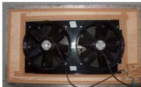
Figure 14: 350mm fans in parallel
