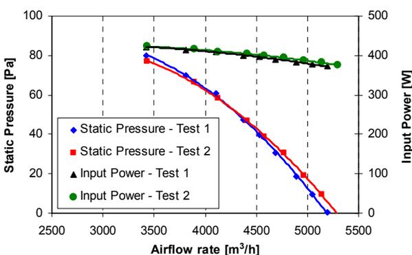
Figure 5: Static pressure and input power vs. airflow rate (450mm fan)
