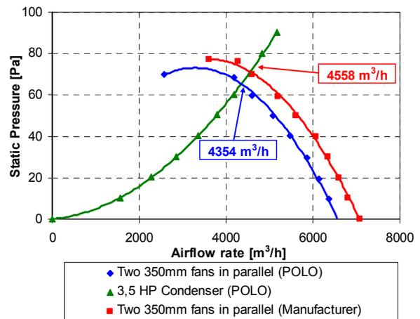
Figure 20: Operation point (3.5HP unit)
