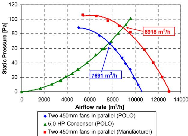
Figure 19: Operation point (5.0HP unit)
