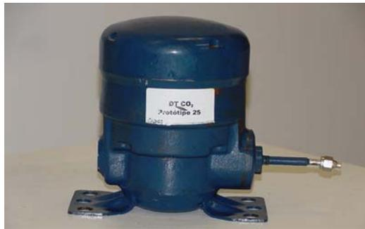
Figure 5. CO<sub>2</sub> compressor
