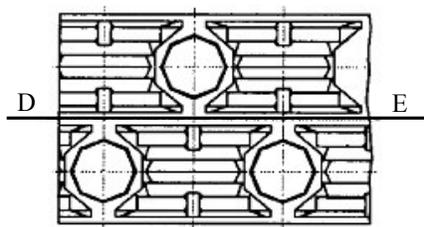
Figure 4: Simple scheme of the investigated fin type
