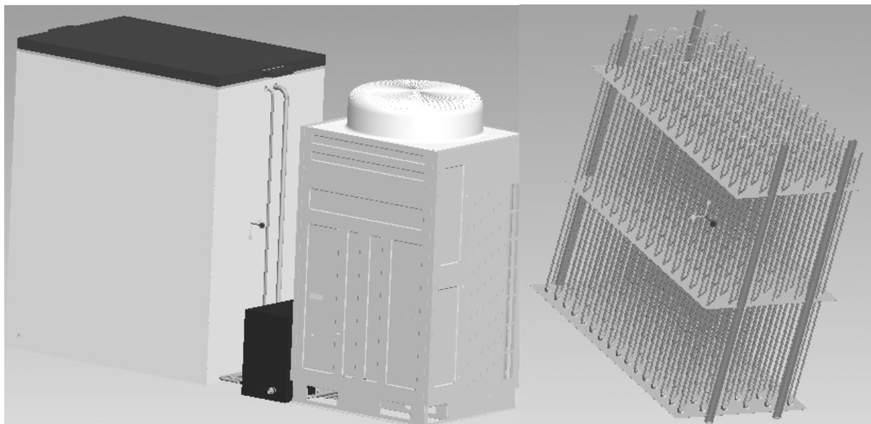
Figure 3: Lay of the whole sub-cooled VRV ice-storage system and the evaporating coils of the ice-storage tank
