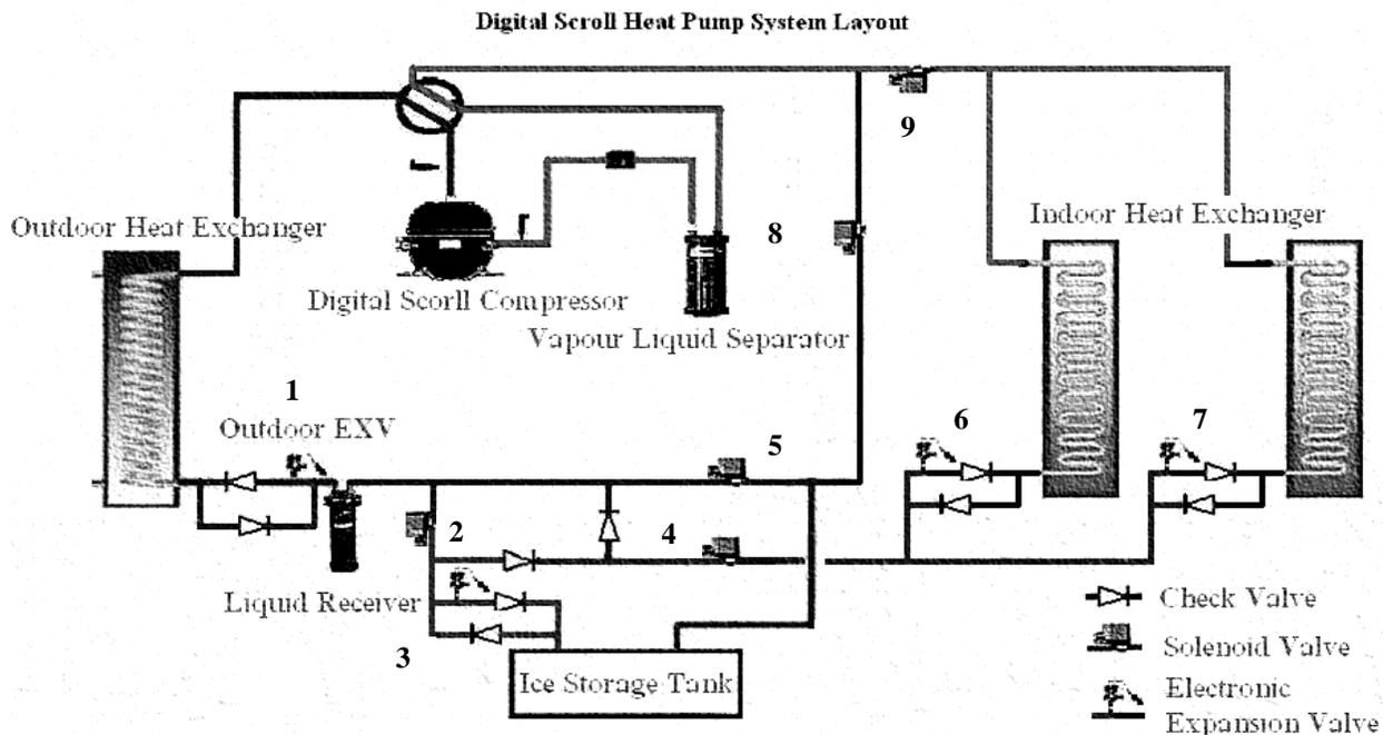
Fig.2: Schematic diagram for the new type sub-cooled ice storage multi-connected system
