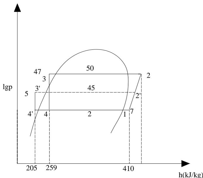
Fig.1 The log p-h schematic diagram of the sub-cooling system
