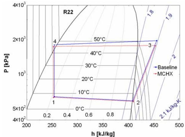
Figure 6 Cycles in P-h Diagram
