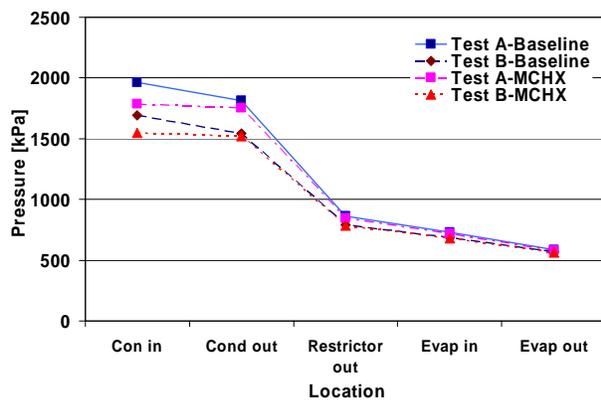
Figure 7 Comparison of Cycle Pressures
