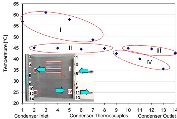
Figure 5 Average Surface Temperatures of Microchannel Condenser
