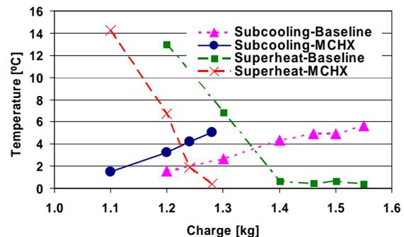
Figure 4 Degree of Superheating and Subcooling vs. Refrigerant Charge Amount
