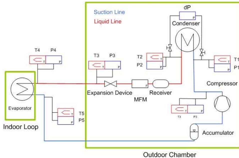
Figure 1 Schematic of Test Set-Up
