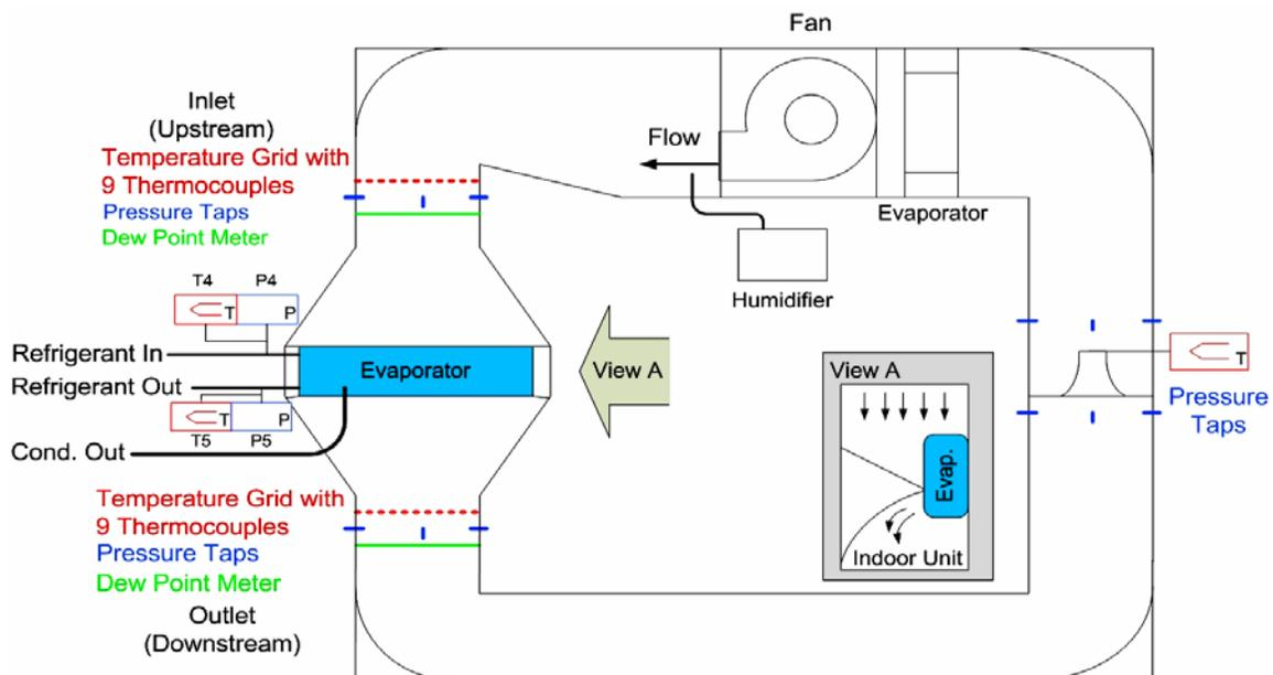
Figure 2 Details of Indoor Loop
