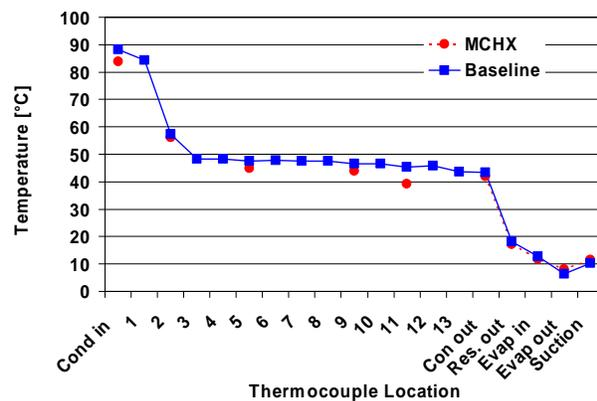
Figure 8 Comparison of Cycle Temperatures
