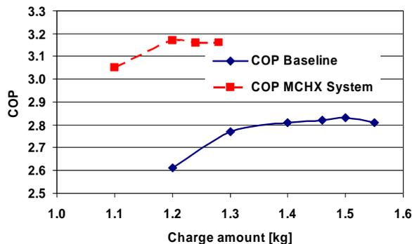
Figure 3 COP vs. Refrigerant Charge Amount
