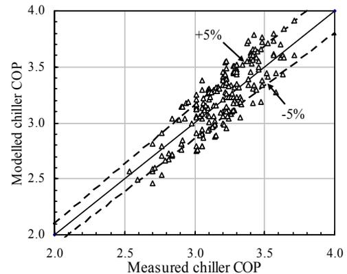
Figure 3: Comparison between the modelled and measured results of chiller COP
