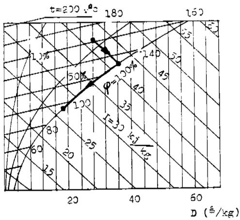
Fig.3 heat transfer process on  $i$ -- $D$  diagram
