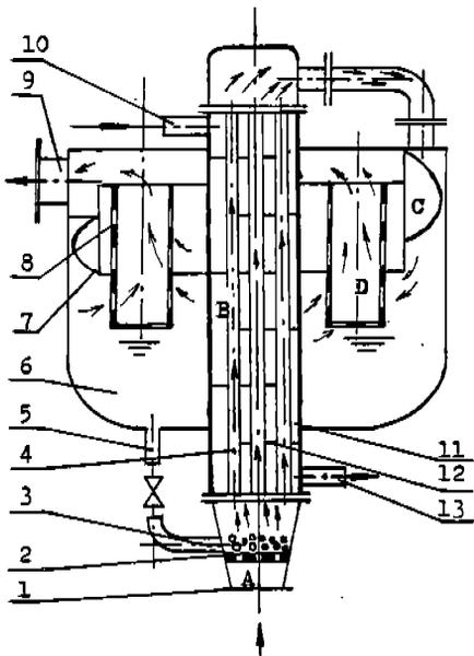
Fig. 1 construction of the cooler
