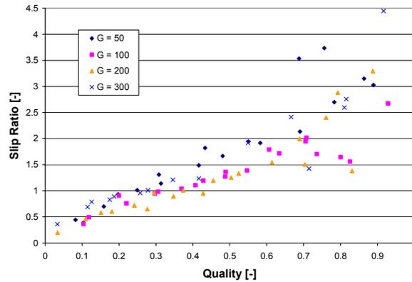
Figure 2: Slip ratio of carbon dioxide in a 14-port microchannel
