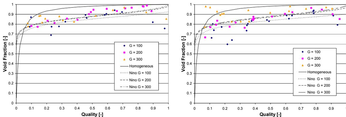
Figure 3: Void fraction of ammonia in (left) a 6-port microchannel and (right) a 14-port microchannel.
