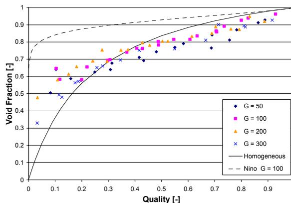
Figure 1: Void fraction of carbon dioxide in a 14-port microchannel.
