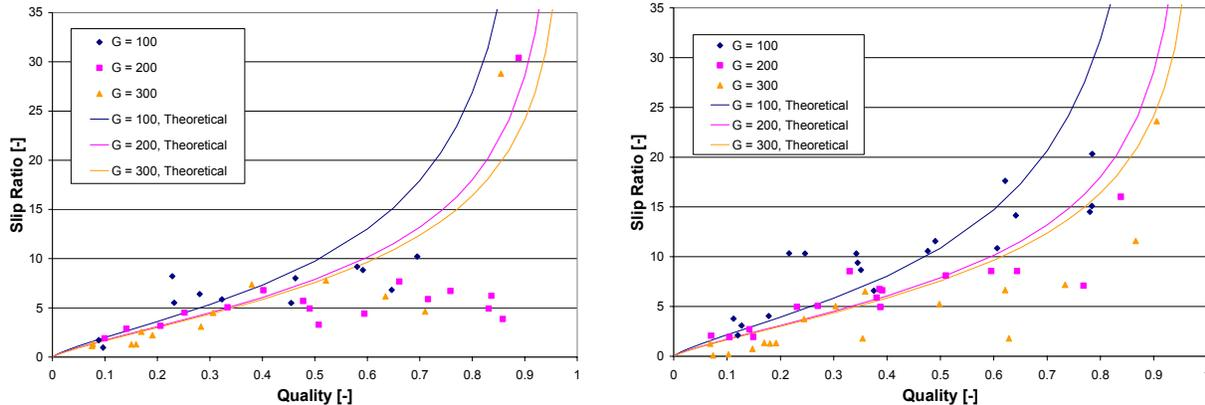
Figure 4: Slip ratio of ammonia in (left) a 6-port microchannel and (right) a 14-port microchannel
