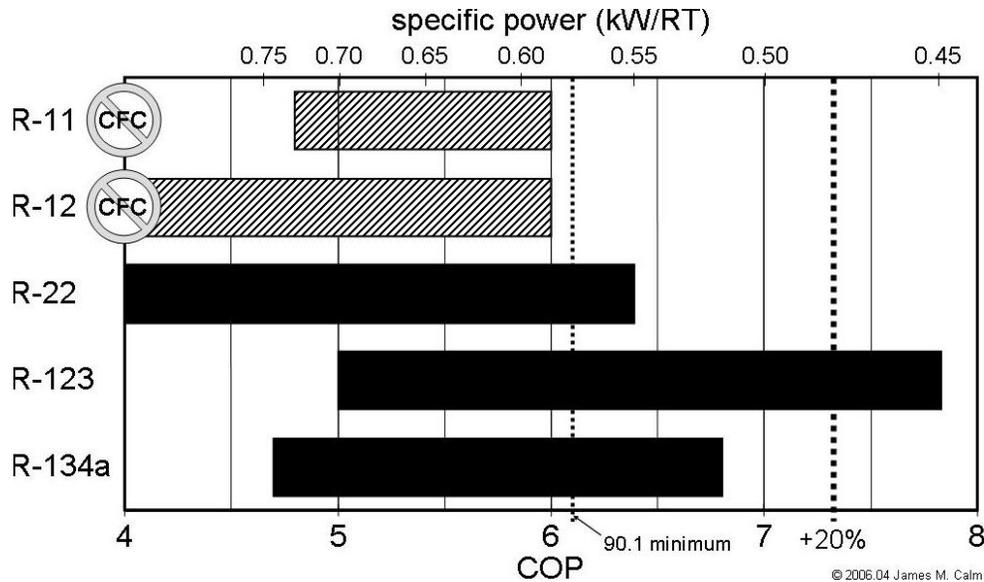
**Figure 3: Efficiency ranges by refrigerant in centrifugal chillers**
