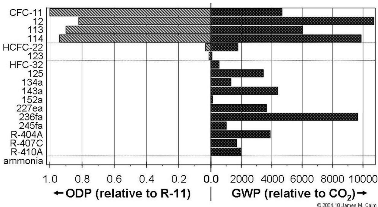
**Figure 2: Ozone depletion potential (ODP) contrasted to global warming potential (GWP) for key refrigerants (based on data from IPCC 2001; WMO, 2003; and Calm and Hourahan, 2001). CFCs generally have high ODP and GWP. HCFCs generally have much lower ODP and GWP. HFCs offer near-zero ODP, but some have very high GWPs.**
