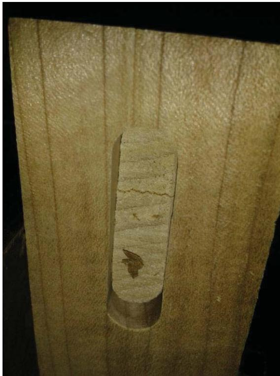
Failure on the T-shaped dowel joints
