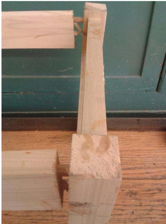
Failure on the stools with glued round mortise and tenon joints.
