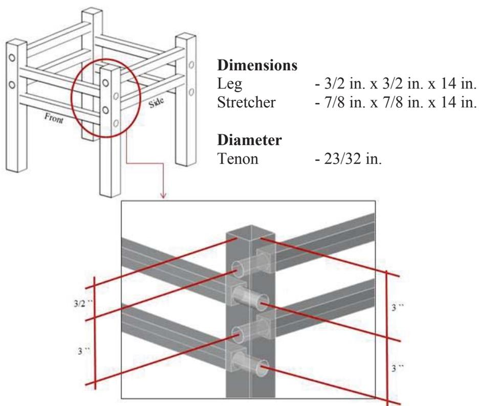
Figure 3-8: Two stretchers glued round mortise and tenon joint frame construction configuration.
