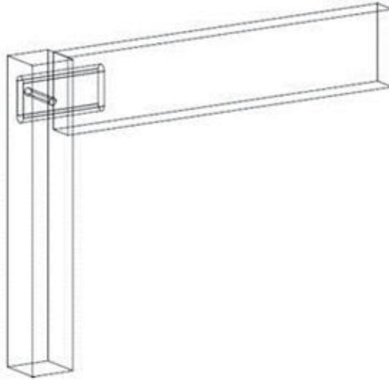
Figure 3-16: Pinned rectangle mortise and tenon L-joint configuration.
