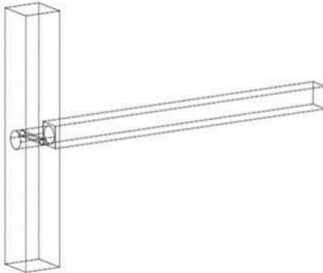
Figure 3-15: Pinned round mortise and tenon T-joint configuration.
