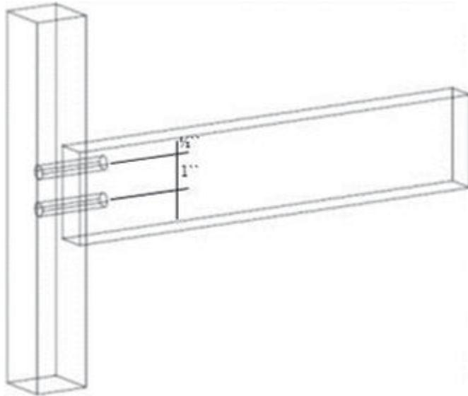
Figure 3-17: Dowel T-joint configuration.
