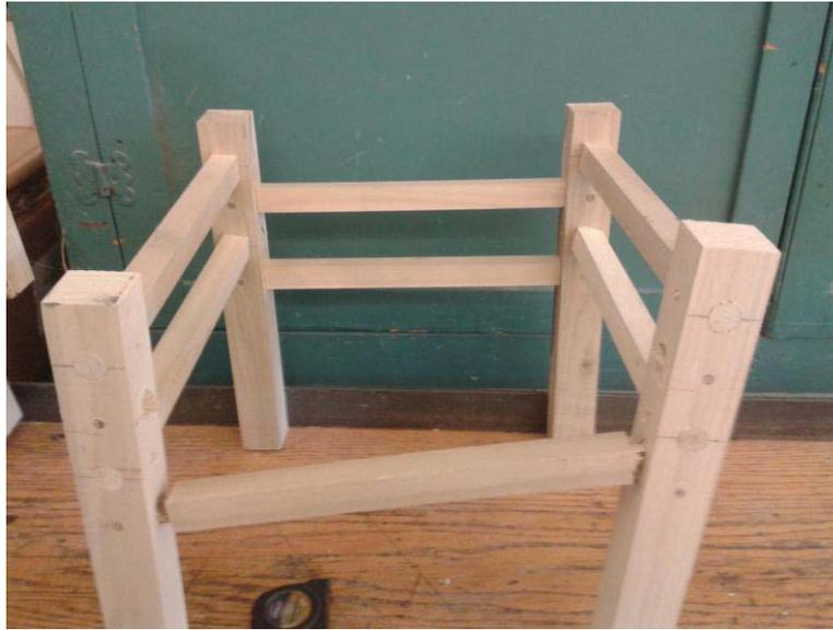
Failure on the stools with pinned rectangular mortise and tenon joints.
