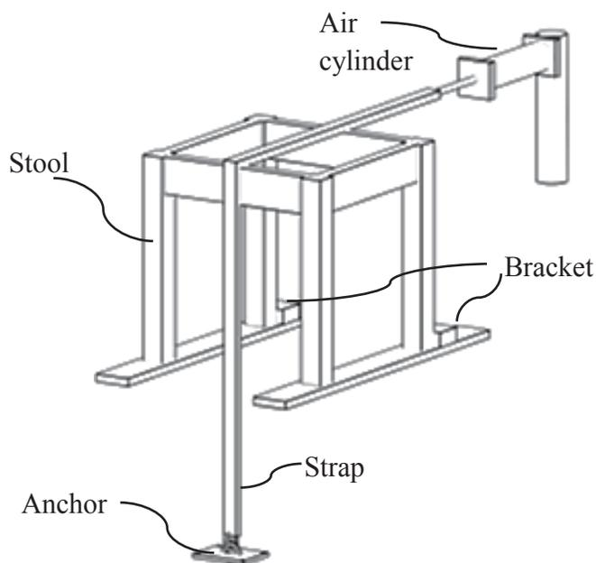
Figure 3-22: Cyclic front-to-back load test configuration.
