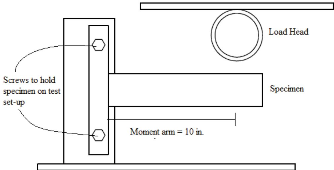
Figure 3-21: Static load test set up.
