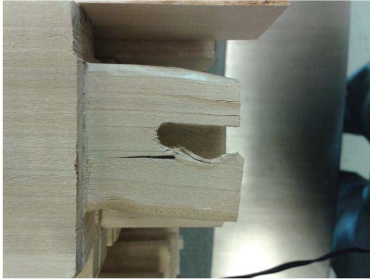
Failure on the stools with dowel joints.
