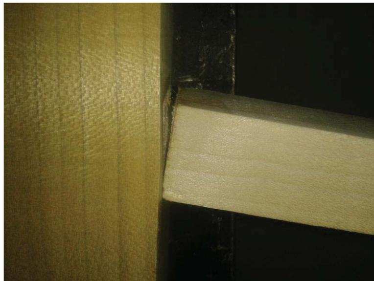
Failure on the L-shaped glued rectangular mortise and tenon joints
