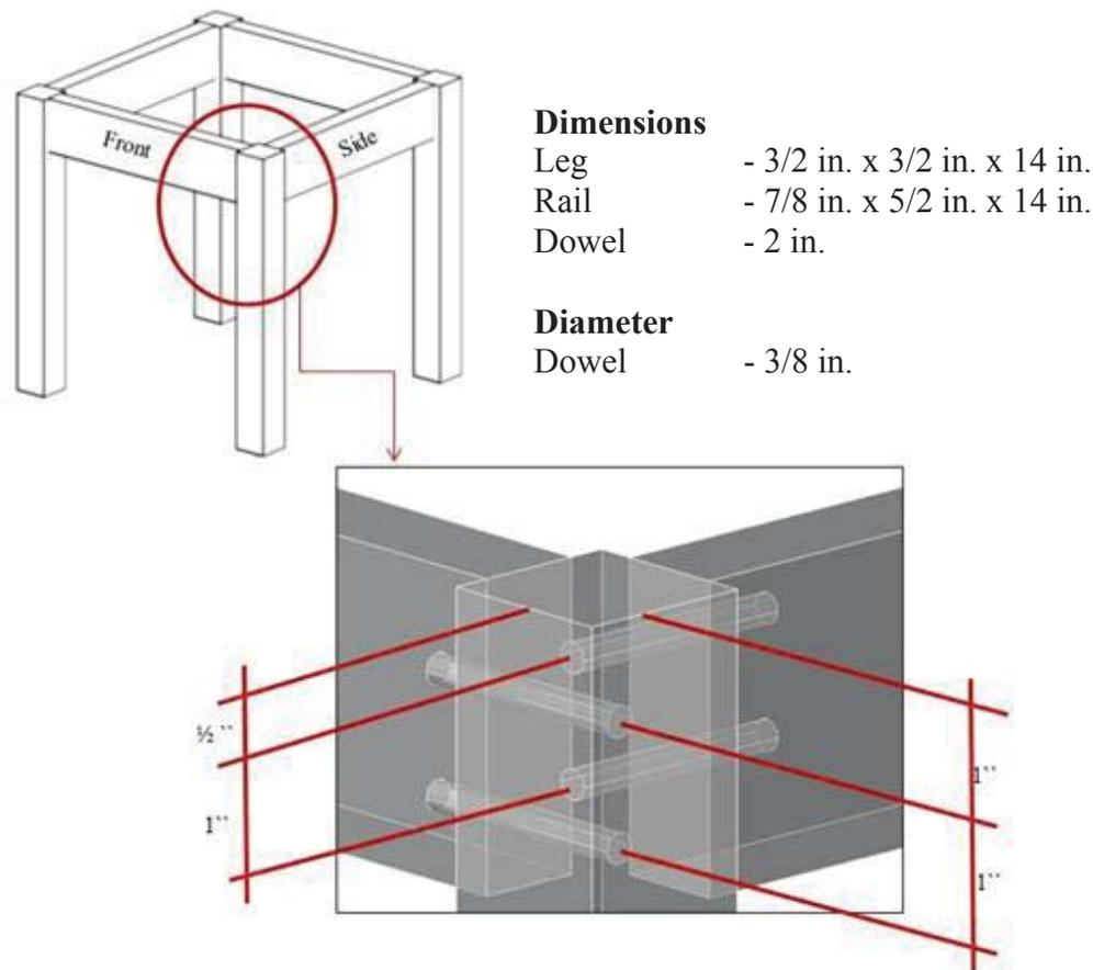
Figure 3-11: Dowel joint frame construction configuration
