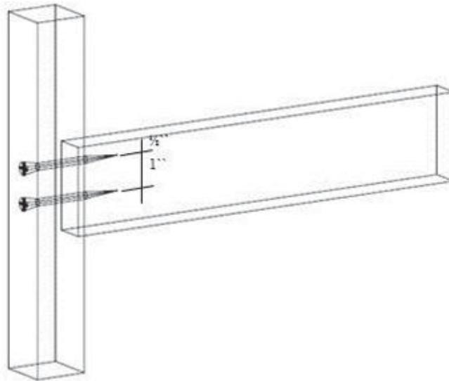
Figure 3-13: Screw T-joint configuration.
