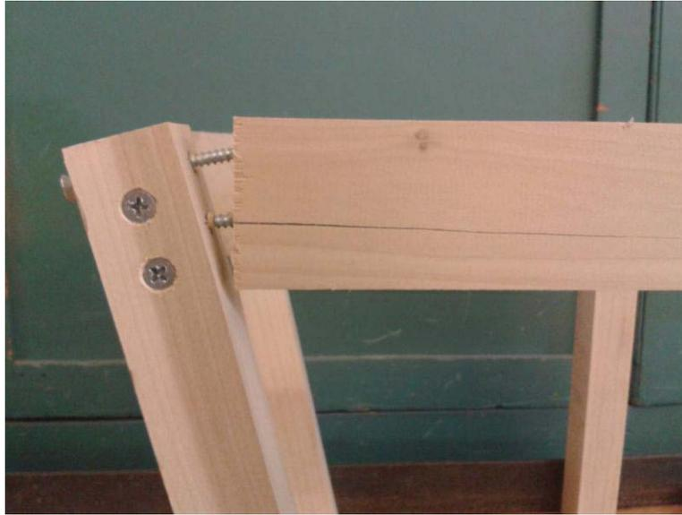
Failure on the stools with bed bolts (with dowel nuts) joints.
