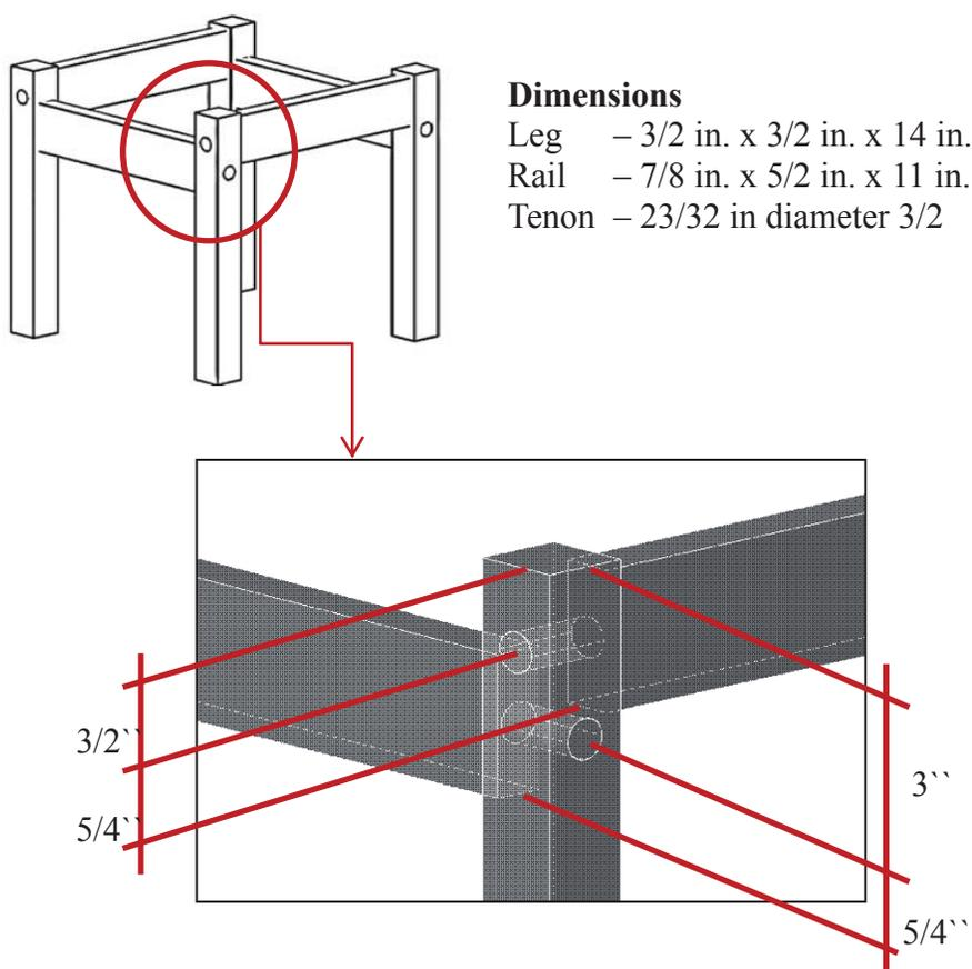
Figure 3-12: Glued round mortise and tenon joint, single rail frame construction
