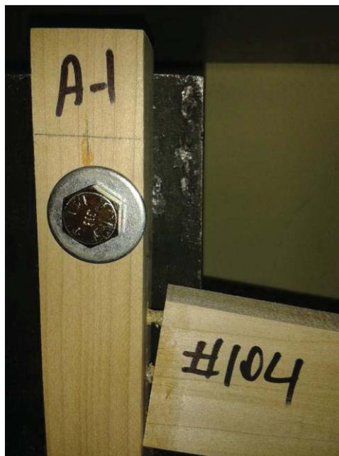
Failure on the T-shaped bed bolts (with dowel nuts) joints
