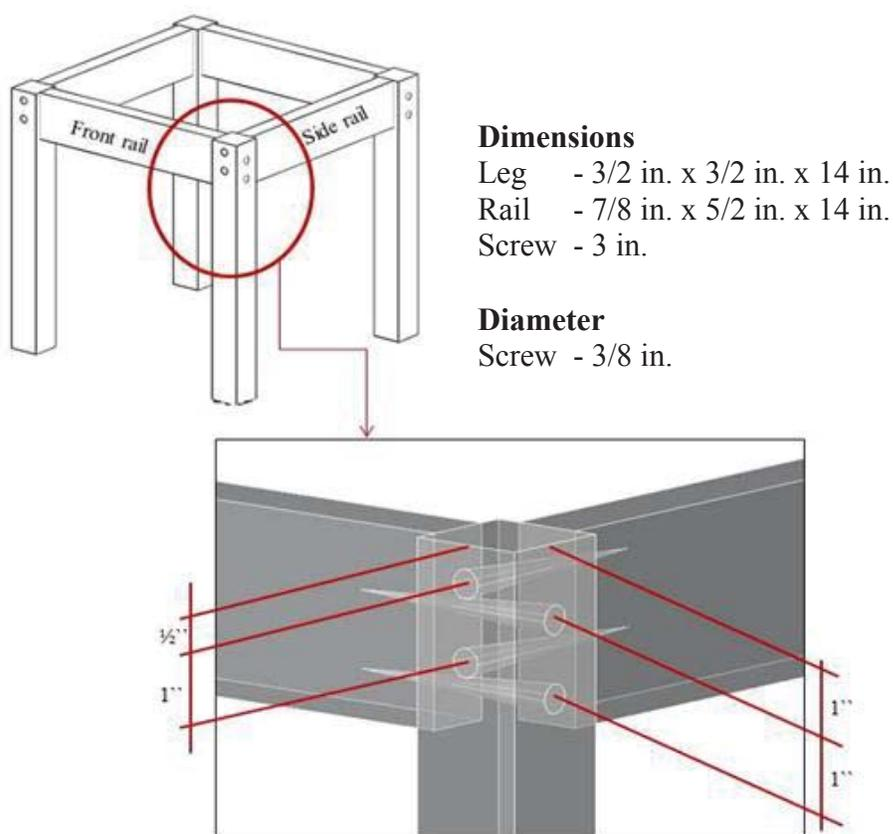
Figure 3-5: Screw joint frame construction configuration.
