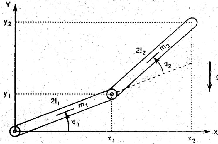
Figure 1. The Two Link Planar Manipulator.
