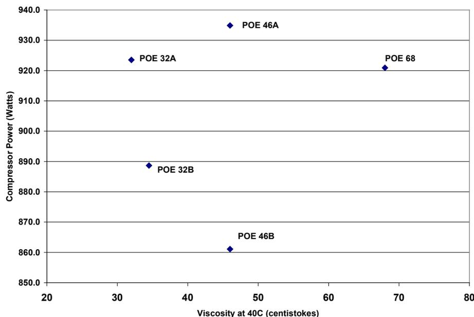
Figure 1: Compressor Power Versus Viscosity for R407C/POE
