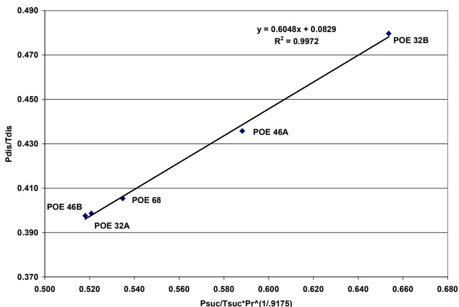
Figure 5: Pd/Td Versus Ps/Ts\*Pr^(1/1.05) – Cooling A
