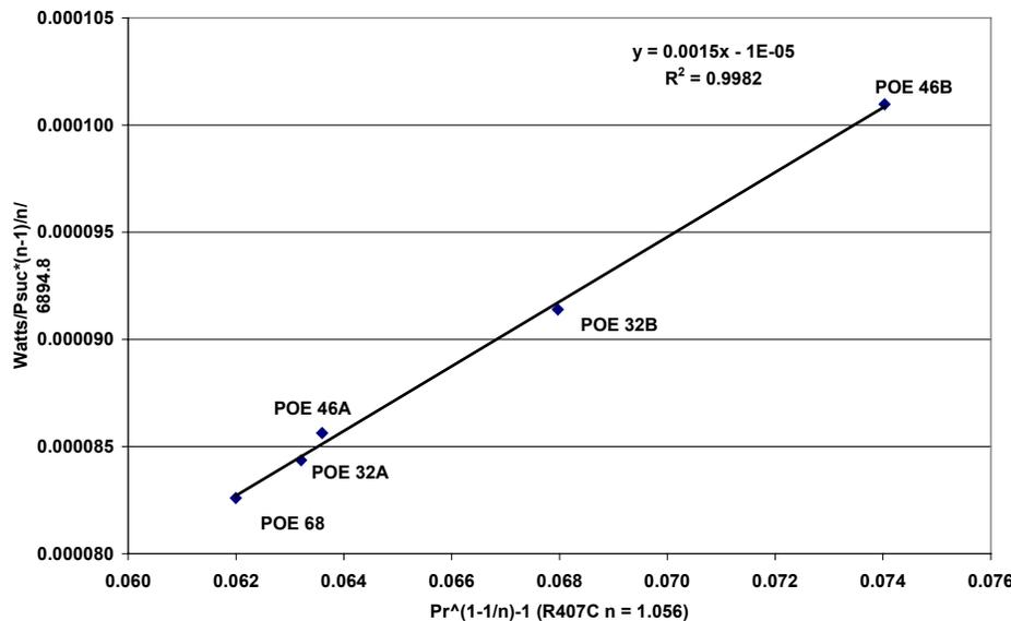
Figure 2: Compressor Work Using Polytropic Analysis – Cooling A
