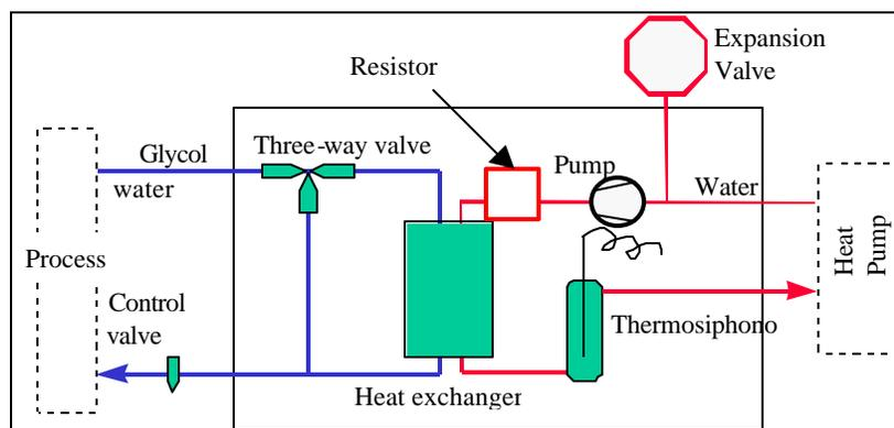
Figure 3: View of the thermal load maker (or Vulcatherm)
