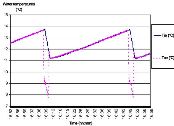
Figure 5: Inlet and outlet evaporator temperatures, 11 l/kW inertia, dead-band 1 K, thermal load 0.4 kW
