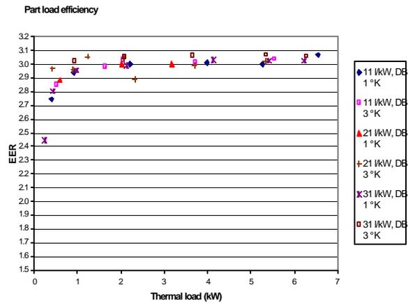
Figure 8: Part load efficiency without sleep power consumption, for various inertia and DB
