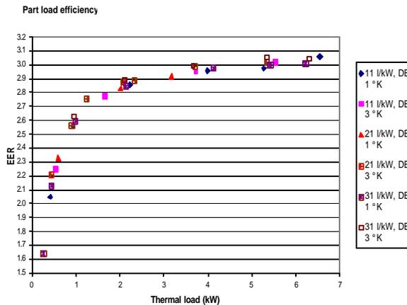
Figure 7: Part load efficiency for various inertia and DB
