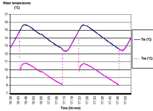
Figure 6: Inlet and outlet evaporator temperatures, 31 l/kW inertia, dead-band 3 K, thermal load 5.4 kW
