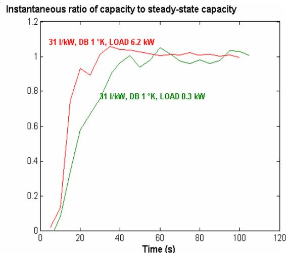
Figure 10: Ratio of the cooling capacity to the steady-state capacity at starting for the series [31 l/kW, DB 1 K]
