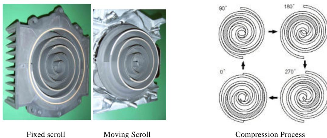
Figure 1: Scroll compressor and compression process (reverse process is expansion)
