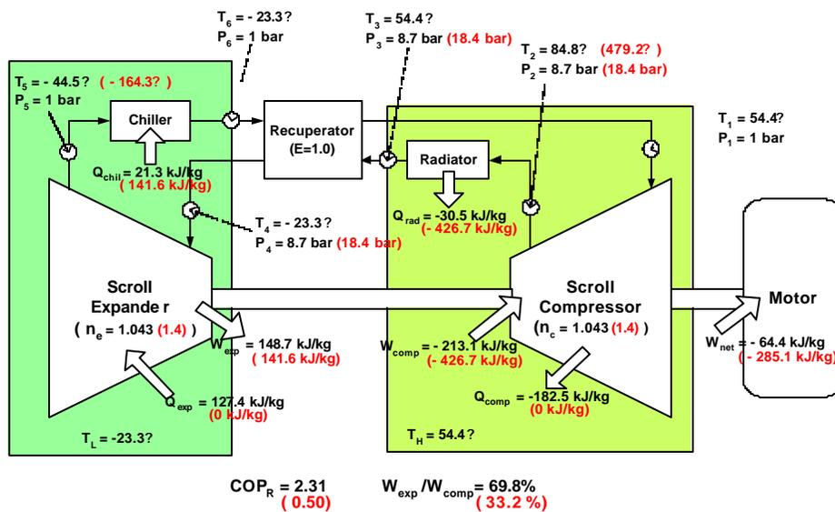
Figure 15: Scroll-type reverse Ericsson cycle refrigerator in comparison with reverse Brayton cycle ( $R_c=8, R_e=8$ )
