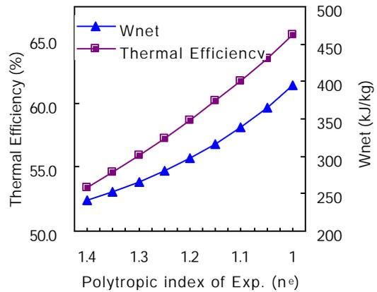
Figure 9: Cycle efficiency and Wnet versus  $n_e$  ( $n_c=1.043$ )
