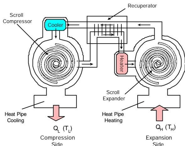
Figure 2: Scroll-type Ericsson cycle for heat engine
