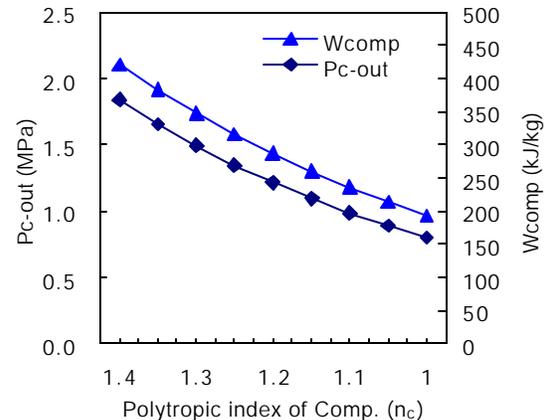
Figure 7:  $P_{c-out}$  and  $W_{comp}$  versus  $n_c$  ( $R_c=8$ )
