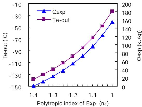
Figure 13:  $T_{e-out}$  and  $Q_{exp}$  versus  $n_e$  in reverse Ericsson refrigerator
