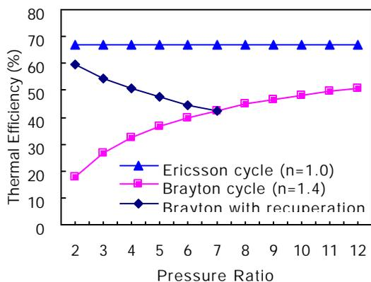
Figure 4: Thermal efficiency versus pressure ratio
