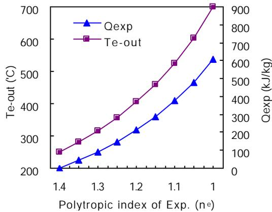
Figure 8: Te-out and Qexp versus  $n_e$
