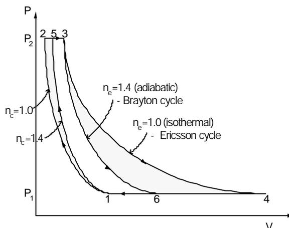
Figure 3: Brayton cycle and Ericsson cycle (P-V diagram)
