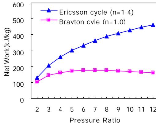
Figure 5: Net work (kJ/kg) versus pressure ratio
