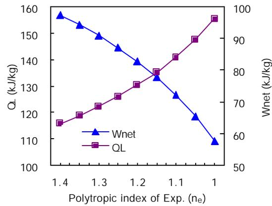
Figure 14:  $Q_L$  and  $W_{net}$  versus  $n_e$  in reverse Ericsson refrigerator
