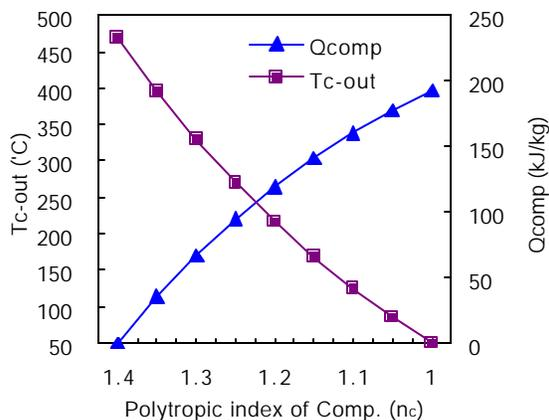
Figure 6:  $T_{c-out}$  and  $Q_{comp}$  versus  $n_c$  ( $R_c=8$ )
