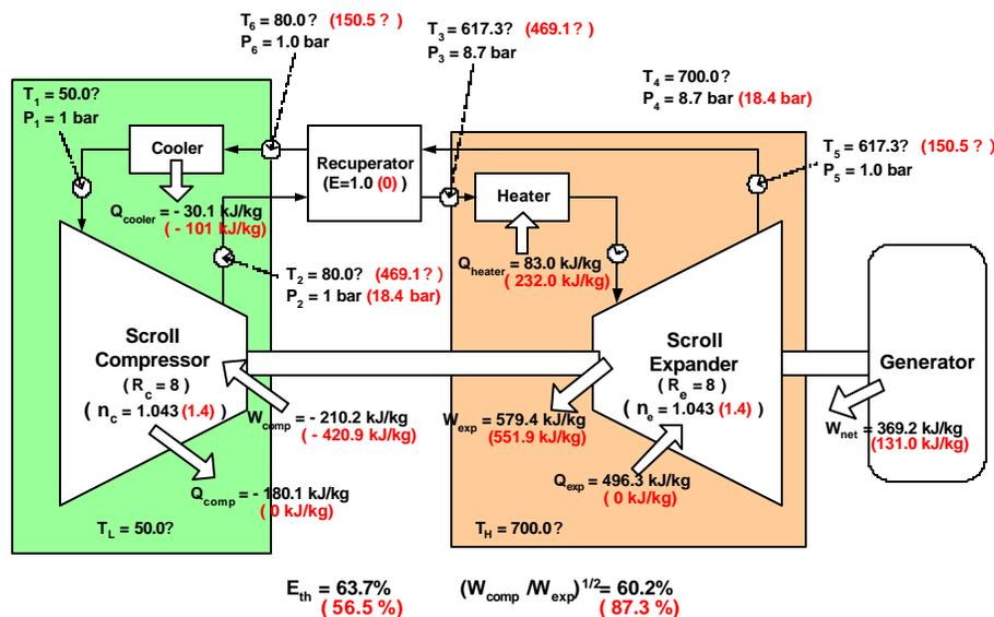
Figure 10: Scroll-type Ericsson cycle engine in comparison with Brayton cycle ( $R_c=8, R_e=8$ )
