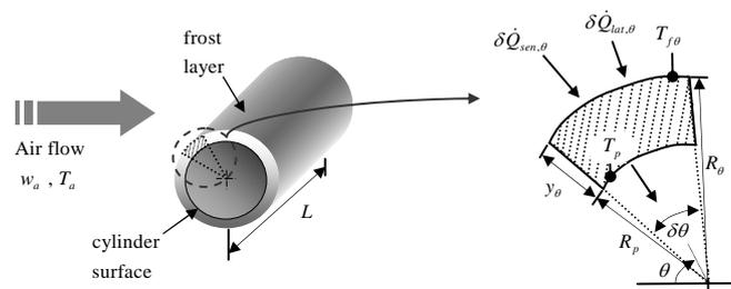
Figure 1: Schematic diagram of frosting formation on a cylinder surface
