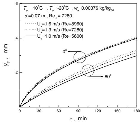
Figure 6: The effect of Reynolds number on the frost thickness at the stagnation and separation points
