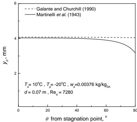
Figure 2: Variation of the frost thickness along the angular coordinate with correlations
