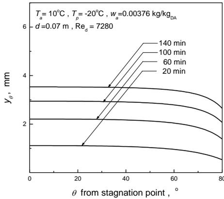
Figure 5: Variations of the frost thickness along the angular coordinate for different times
