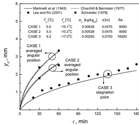
Figure 3: Comparisons of numerical results and experimental data on the frost thickness
