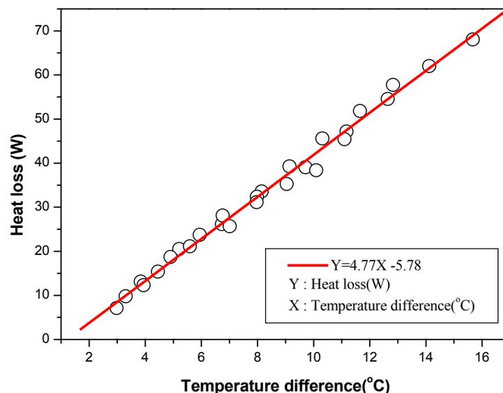
Figure 3. Relationship between temperature difference and heat loss
