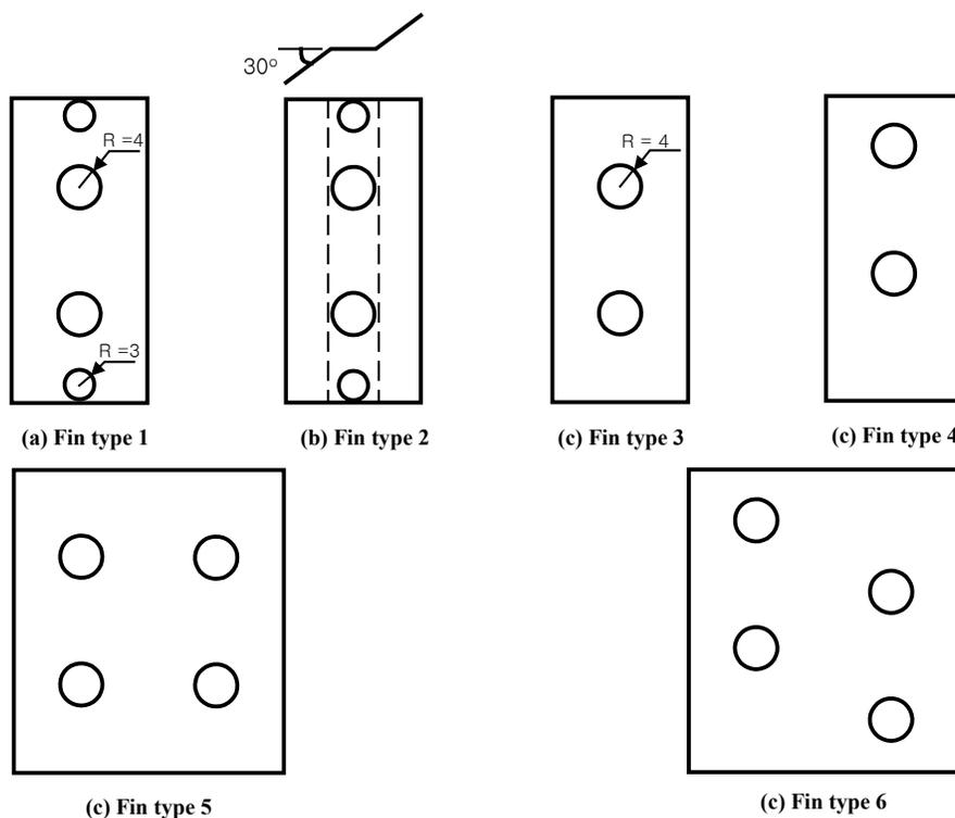
Figure 2. Fin configurations of the evaporator coil
