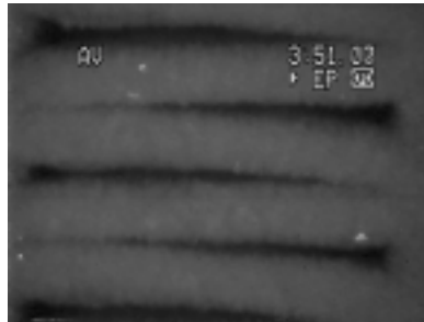
Figure 2: Frost image recorded by focusing a CCD camera on the front view of the heat exchanger
