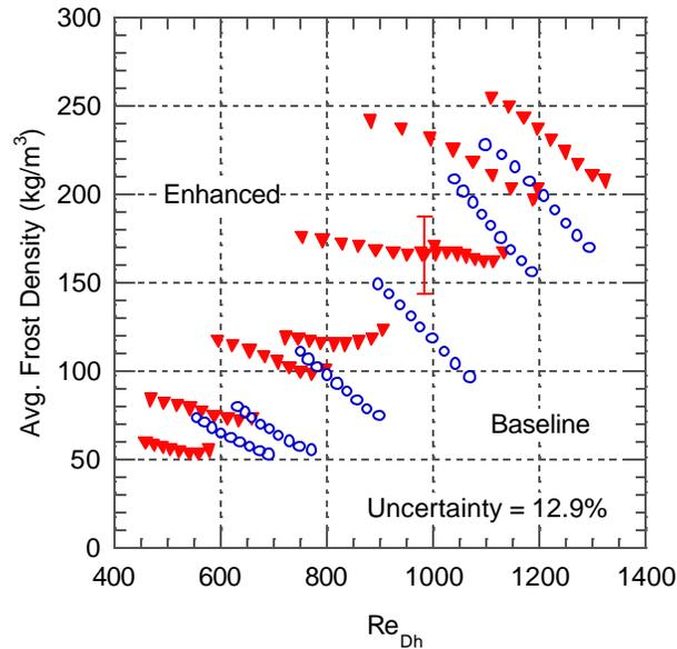
Figure 6: Frost density calculated from mass deposition rate data
