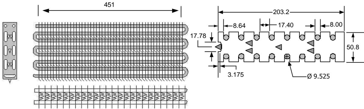
Figure 1: Heat exchanger geometry and vortex generator configuration
