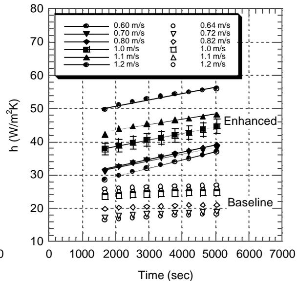
Figure 4: The heat transfer coefficient plotted as a function of face velocity and deposition time.
