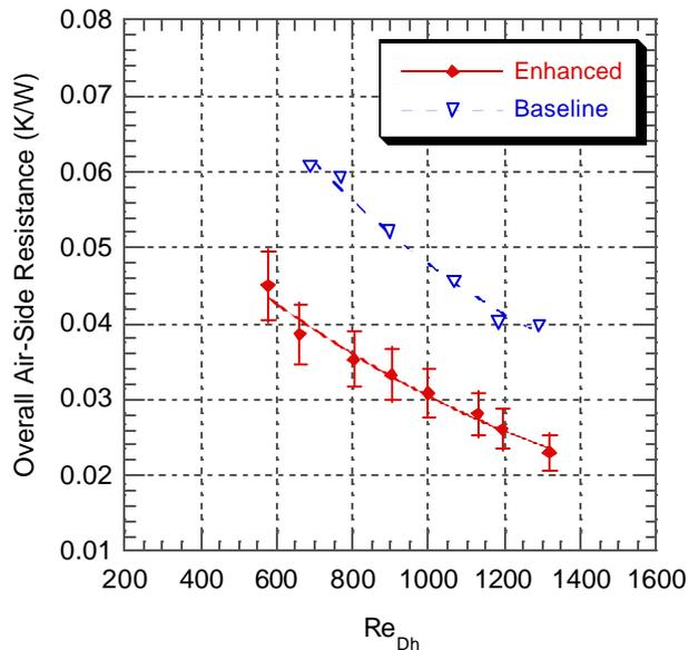
Figure 3: The overall air-side thermal resistance is 35% to 42% lower for the enhanced evaporator.
