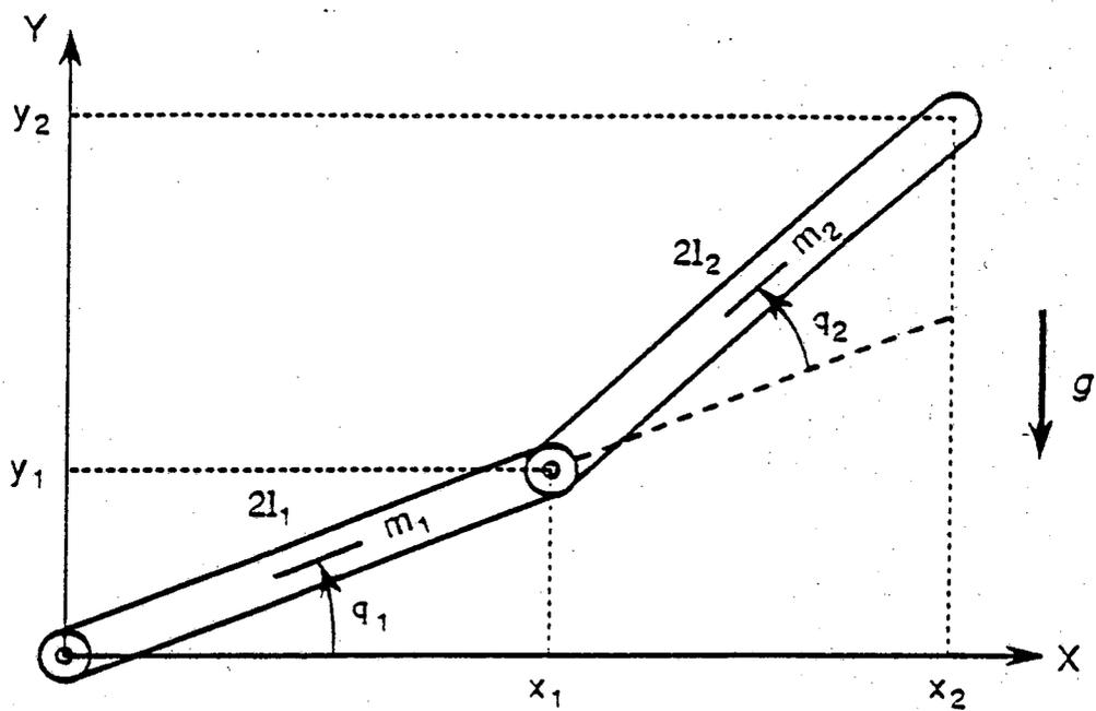
Figure 1. The Two Link Planar Manipulator.
