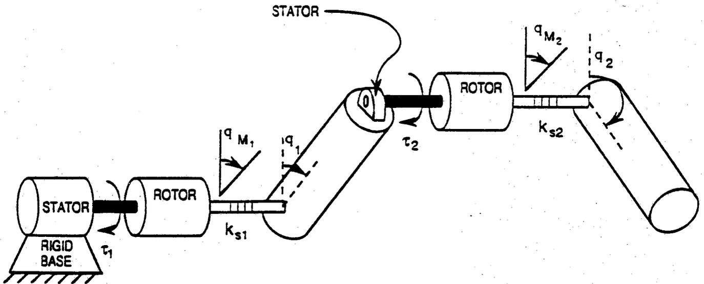
Figure 2. Conceptual Diagram of Two Link Compliant Manipulator.
