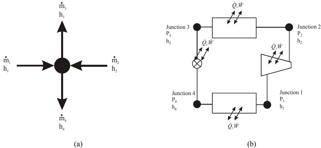
Figure 2: A VapCyc Diagrams (a) VapCyc Junction, (b) Simple Refrigeration Cycle
