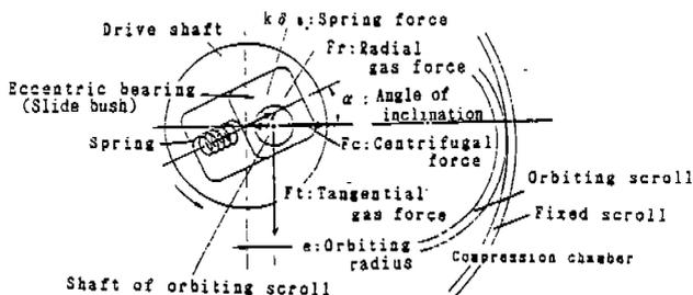
Fig.4 Slide-bushing mechanism
