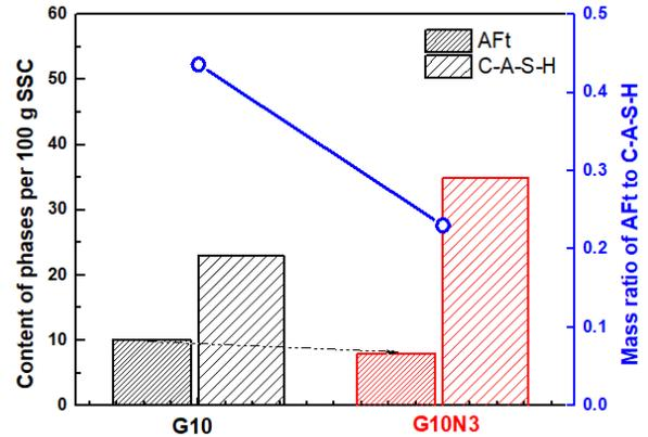
Figure 5. Amount of AFt and C-A-S-H phase in SSC with and without nano SiO<sub>2</sub> at 28 days.
