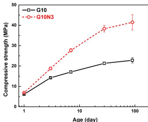
**Figure 1.** Compressive strength of SSC with and without nano  $\text{SiO}_2$  as a function of time.
