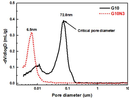
Figure 4. Pore size distribution of SSC with and without nano SiO<sub>2</sub> at 90 days.
