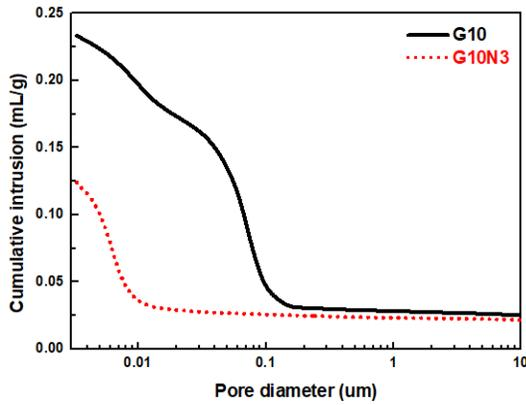
Figure 3. Porosity of SSC with and without nano SiO<sub>2</sub> at 90 days.
