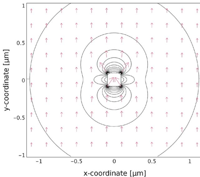
**Fig. 1** The calculated magnitude and direction of the electric field of the predominantly  $y$ -polarized  $E^{(0,1)}$  mode propagating along a  $180 \text{ nm} \times 180 \text{ nm}$  gold wire embedded in a dielectric cladding. The  $x$ -polarized  $E^{(1,0)}$  mode is obtained by  $90^\circ$  rotation
