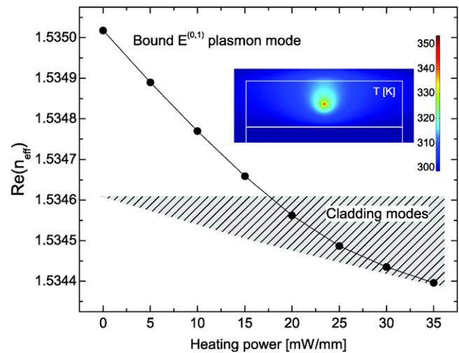
**Fig. 3** The real part of the effective index for the  $E^{(0,1)}$  mode versus electrical heating power for a gold nanowire. The grey area corresponds to the refractive index of the cladding layer which has a temperature-induced index gradient. The calculated temperature profile (color) is shown in the *inset*, corresponding to a heating power of  $20 \text{ mW/mm}$
