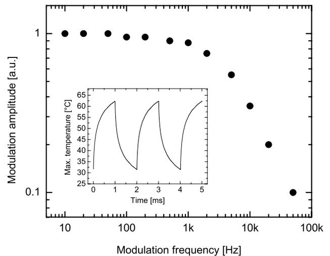
**Fig. 7** Measured frequency response of the plasmonic nanowire attenuator/modulator for a fixed driving voltage amplitude (2 V). The inset shows the simulated temperature transients in the vicinity of the wire for a 0.5 kHz modulation, with the extent of the y-axis corresponding to full modulation
