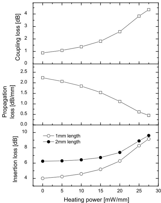
**Fig. 4** Effect of heating on coupling loss and propagation loss in nanowire waveguides. The total insertion loss increases with heating, but the change is considerably smaller than observed in experiment
