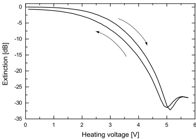
**Fig. 6** Measured thermo-optical memory effect in BCB polymer. A plasmonic VOA heated to achieve  $>30$  dB extinction exhibits a slowly reversible refractive index change when returned to the off-state
