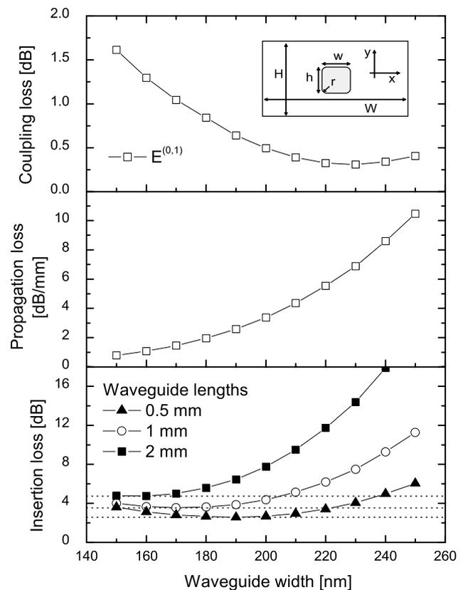
**Fig. 2** Calculated coupling loss, propagation loss and fiber-to-fiber insertion loss for 0.5-, 1- and 2-mm long gold nanowire waveguides in a  $20 \mu\text{m}$  thick cladding layer at  $\lambda = 1550 \text{ nm}$ . Similar values are obtained for both polarizations, so only the  $E^{(0,1)}$  results are shown. The *inset* in the top panel schematically shows the simulated device geometry
