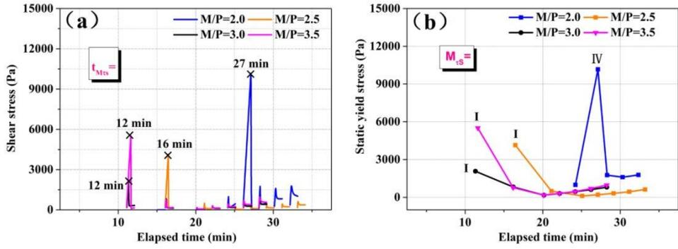
Figure 7. Evolution of (a) shear stress and (b) static yield stress with elapsed time for mixtures with different M/P ratio.
