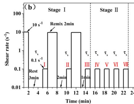
Figure 3. (a) Peak value represents the static yield stress and (b) the testing procedure.
