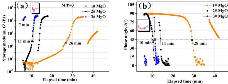
Figure 5. Evolution of (a) storage modulus and (b) phase angle with elapsed time for mixtures with different MgO fineness.
