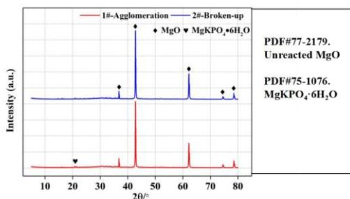
Figure 9. XRD patterns of reversible agglomeration and the broken-up mixture at 10 min age.
