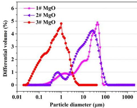
Figure 1. The particle size distributions of magnesia.
