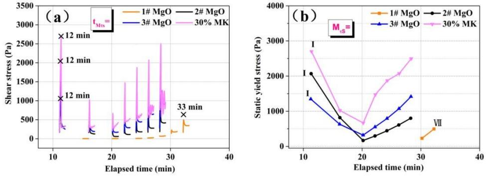
Figure 8. Evolution of (a) shear stress and (b) static yield stress with elapsed time for mixtures with different MgO fineness and 30% MK.
