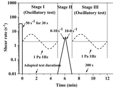
Figure 2. The time sweep testing procedure.
