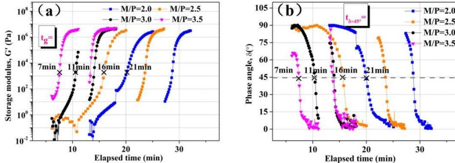
**Figure 4.** Evolution of (a) storage modulus and (b) phase angle with elapsed time for mixtures with different M/P ratio.
