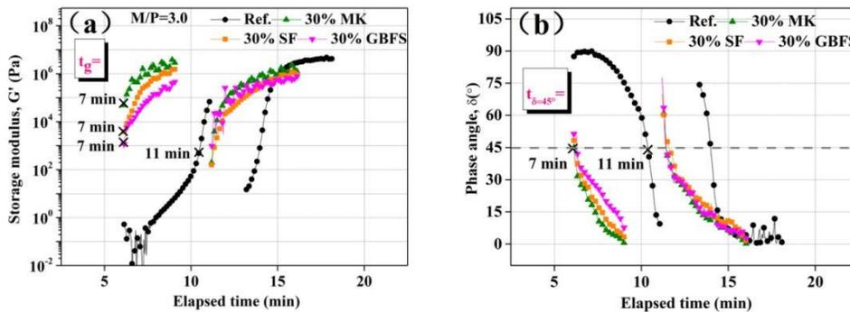
Figure 6. Evolution of (a) storage modulus and (b) phase angle with elapsed time for mixtures with different types of 30% SCMs.
