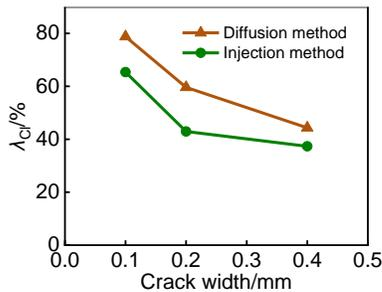
**Figure 9.** The improvement coefficient of chloride aggressive resistance of all specimens
