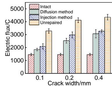
**Figure 8.** Electric flux of test specimens within 6h
