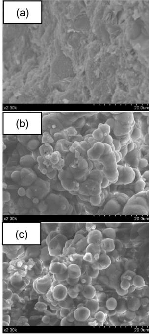
**Figure 6.** Morphology of material in cracks of specimen with initial crack width of 0.1 mm: (a) Unrepaired; (b) Repaired by diffusion method; (c) Repaired by injection method
