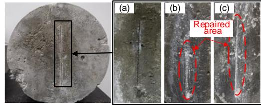
Figure 4. Surface condition of specimen with initial crack width of 0.2 mm repaired by diffusion method: (a) Before repair; (b) Under repair; (c) After restoration
