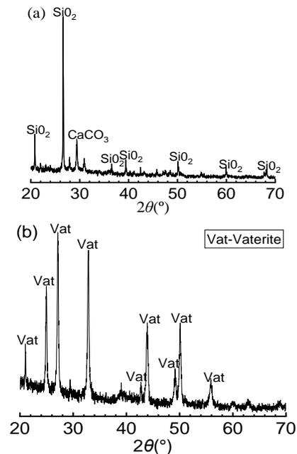
Figure 5. The XRD pattern of the material in the crack of the specimen with the initial crack width of 0.1 mm: (a) Unrepaired; (b) Repaired by diffusion method
