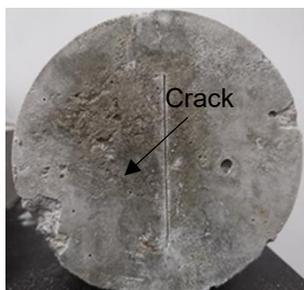
**Figure 1.** Concrete specimen with precast crack
