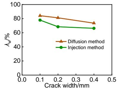
**Figure 7.** The improvement coefficient of the waterproof performance of all specimens
