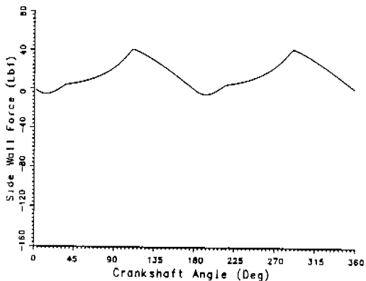
Fig. 6. Side Wall Forces on a Quadro-Flex Double Piston
