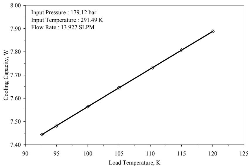
Fig.3 Effect of the load temperature on the cooling capacity
