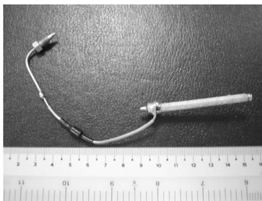
Fig.1a A Hampson-type J-T cryocooler (Xue, 2001) Fig.1b A picture of the Hampson-type J-T cryocooler
