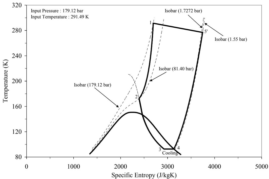
Fig.2 A typical simulated T-s diagram of the Hampson-type Joule-Thomson (J-T) cooler
