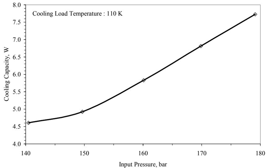
Fig.4 Effect of the input pressure on the cooling capacity
