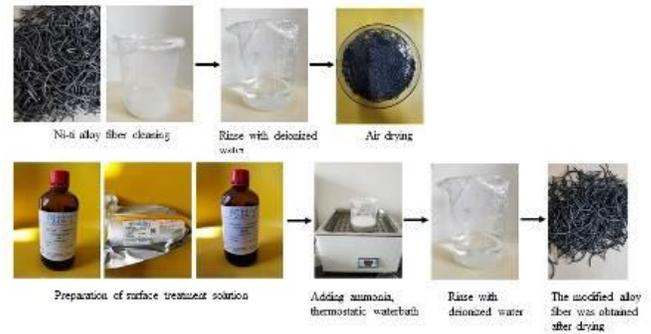
Figure 1. Flow chart of SMA fiber modification
