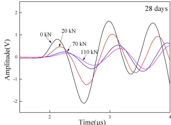
Figure 8. Time domain waveform of different loading stages
