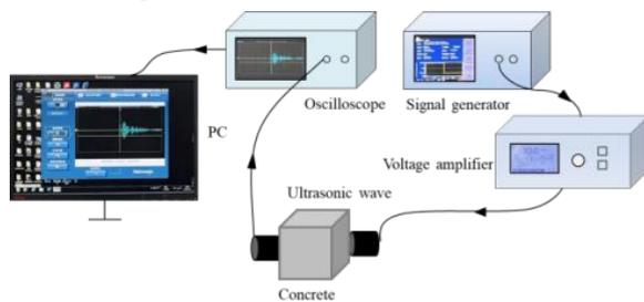
Figure 1. Principle of ultrasonic monitoring
