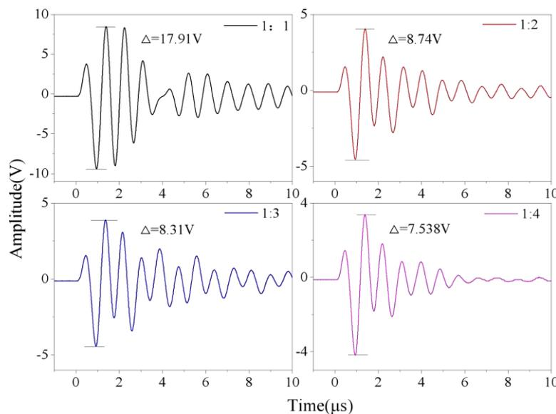
**Figure 6.** Time-domain waveform of different backing ratio
