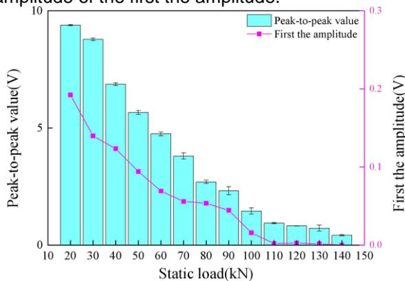
**Figure 9.** Peak-to-peak value and amplitude of first the amplitude in different loading stages
