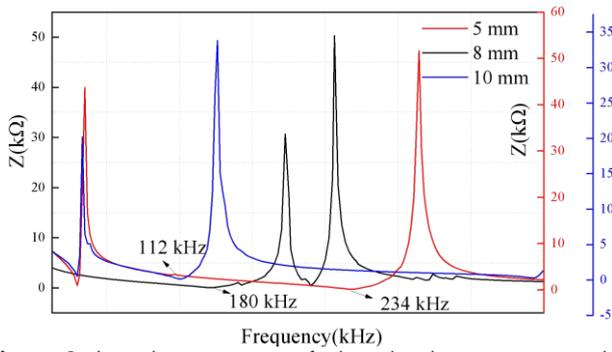
**Figure 3.** Impedance spectra of piezoelectric components with different thickness
