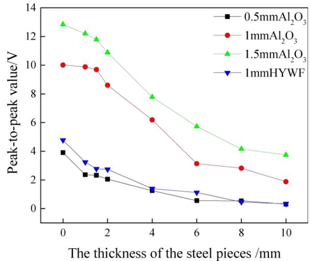
**Figure 5.** Peak-to-peak values of different matching layers
