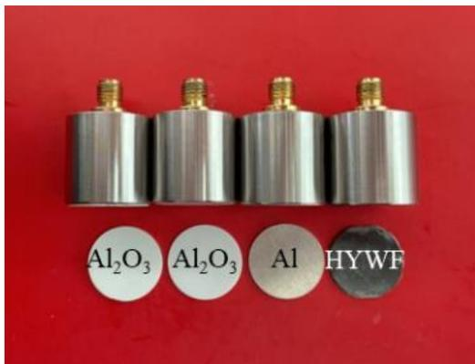
**Figure 4.** Pictures of sensors at different matching layers
