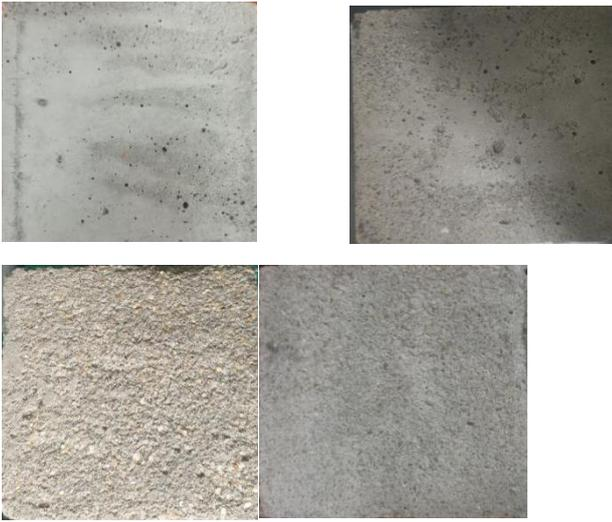
Fig. 2 Concrete surface under different cycles
