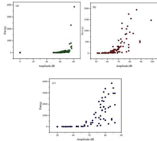
**Fig. 6** Amplitude-energy correlation diagram under different freeze-thaw cycles
