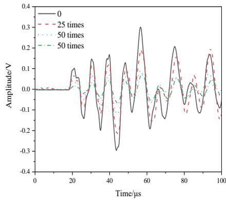
Fig. 4 Amplitude under different number of freeze-thaw cycles
