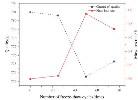
Fig. 3 Mass loss rate under different freeze-thaw cycles
