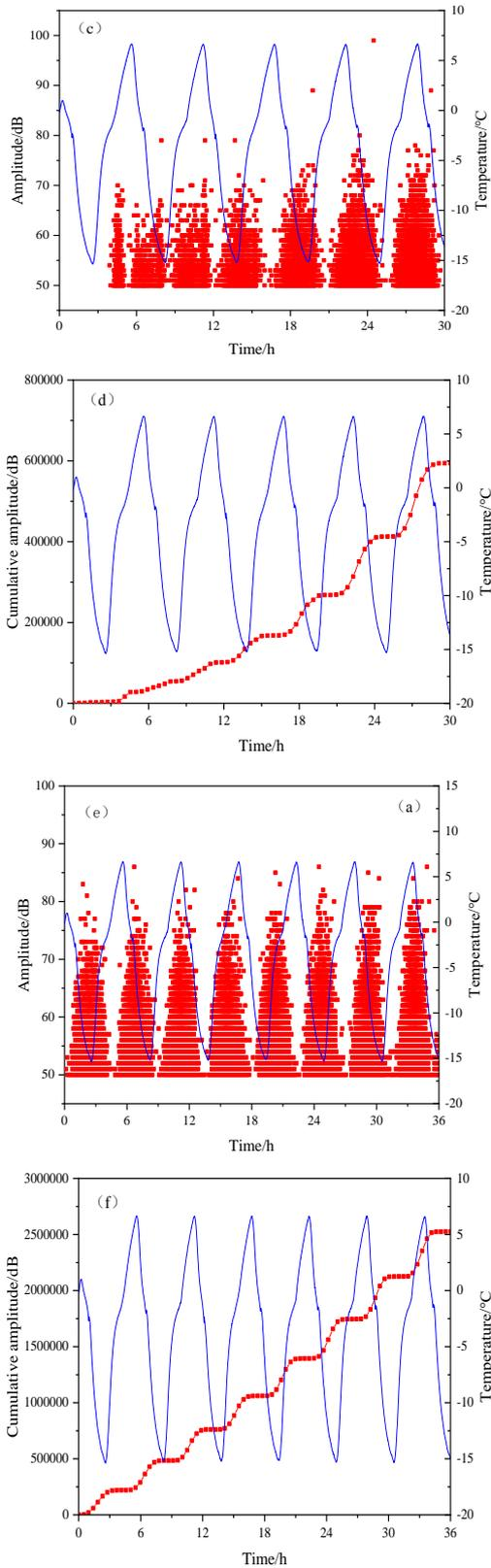
**Fig. 5** (a), (c) and (e) are amplitude and temperature time curves of freezing-thawing cycles 25, 50 and 75 times respectively. (b), (d) and (f) are the cumulative amplitude and temperature time curves of freezing-thawing cycles for 25, 50 and 75 times respectively
