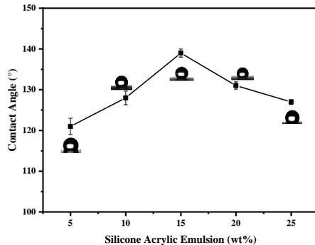
**Figure 2.** Effects of silicone-acrylic emulsion on water contact angle of coating
