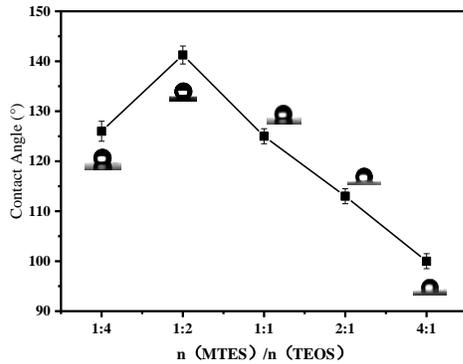
**Figure 4.** Effects of n(MTES)/n(TEOS) on the water contact angle of coating
