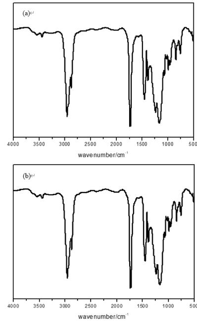
**Figure 3.** FT-IR spectra of (a) silicone-acrylic emulsion and (b) organic-inorganic hybrid super-hydrophobic coating
