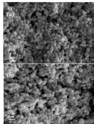
**Figure 6.** SEM of hybrid coating made from (a) content of FAS was 3% (b) content of FAS was 4%
