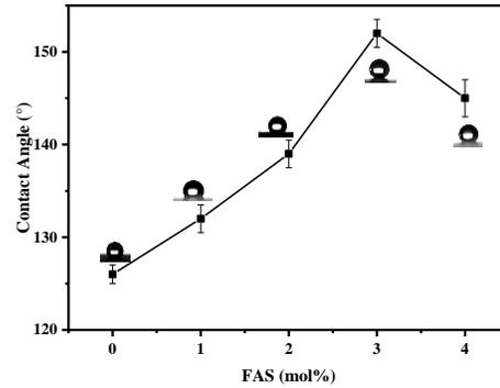
**Figure 5.** Effects of FAS addition amount on the water contact angle of coating
