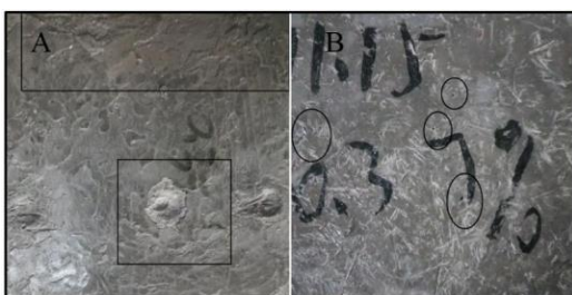
Figure 3. Surface morphology of untreated glass fiber reinforced cement after freeze-thaw cycles.
