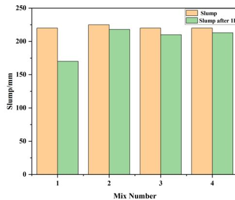
Figure 4. The slump and the slump after 1h of High performance concrete.
