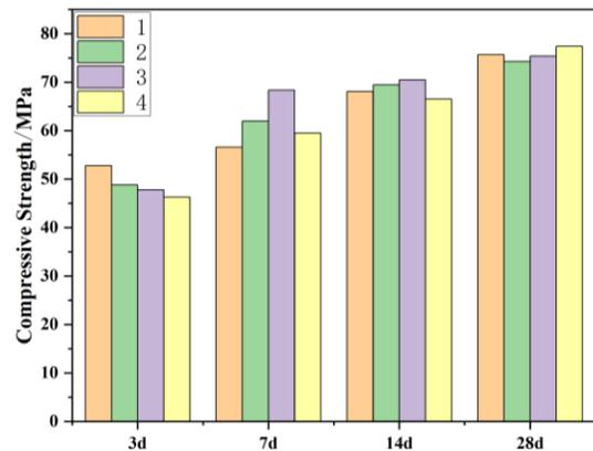
Figure 3. Compressive strength of high performance concrete.
