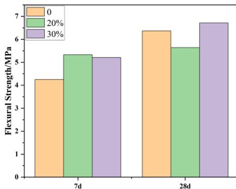
Figure 2. Flexural Strength of hard concrete.
