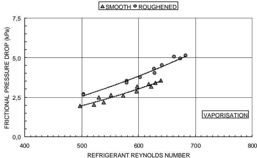
Figure 7: Frictional pressure drop vs. refrigerant Reynolds number under experimental tests.
