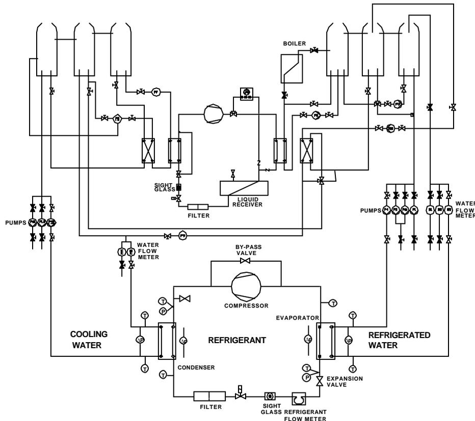
Figure 3: Schematic view of the experimental test rig
