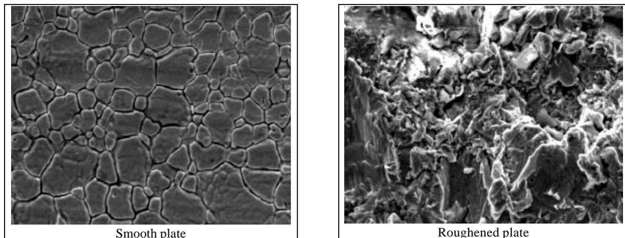
Figure 2: Smooth and roughened surface at the scanning electron microscope (1200 x)
