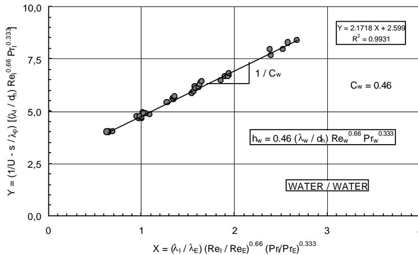
Figure 4: Modified Wilson plot results for calibration of water side heat transfer coefficient.
