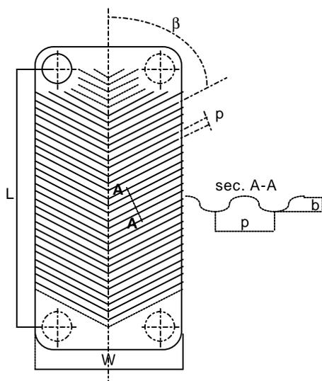
Figure 2: Schematic view of the plate
