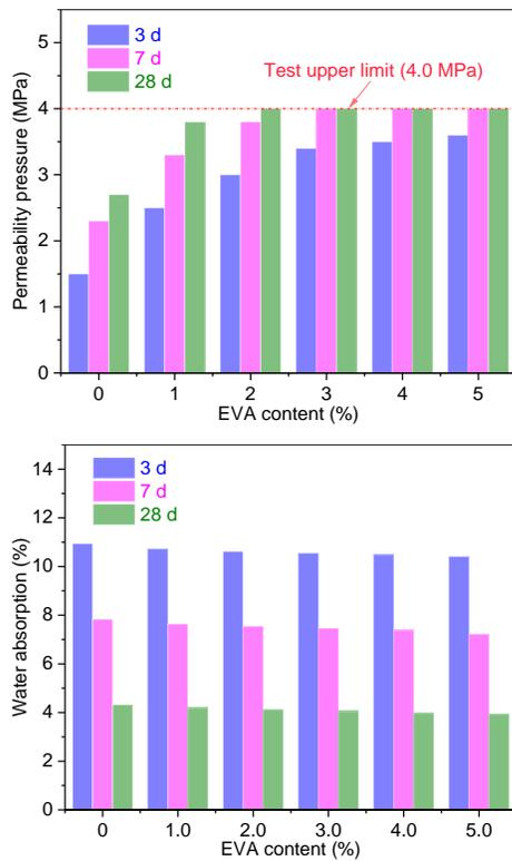
**Figure 3.** Impermeability pressure and water absorption of EVA powder modified CSA cement waterproof repair mortar
