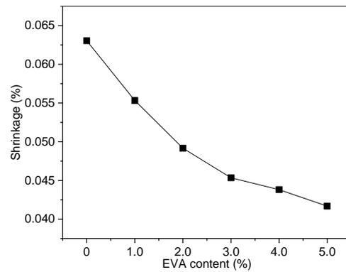
**Figure 6.** Shrinkage of EVA powder modified CSA cement waterproof repairing mortar
