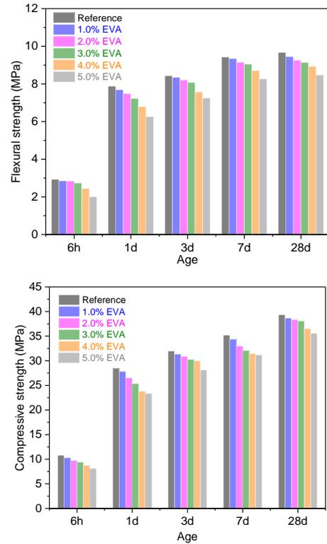
**Figure 4.** Flexural strength and compressive strength of EVA powder modified CSA cement waterproof repair mortar
