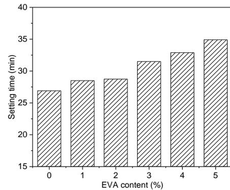
**Figure 2.** Setting time of EVA powder modified CSA cement waterproof repair mortar
