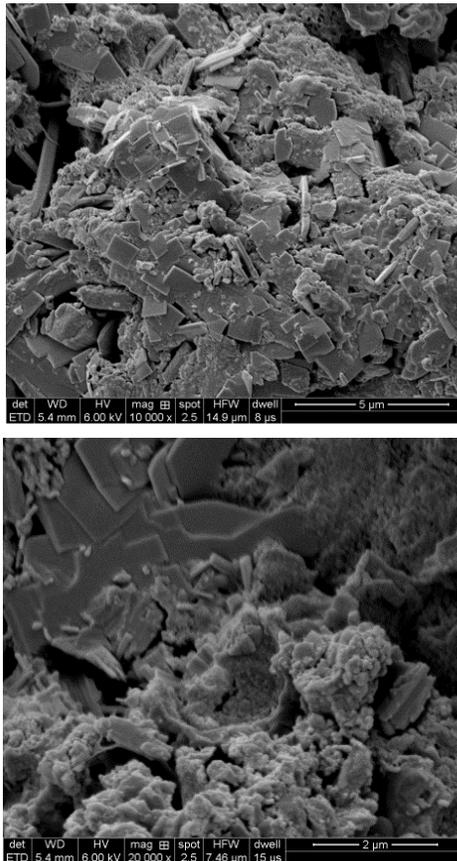
**Figure 8.** Morphology of EVA in the hardened CSA cement repair mortar at the hydration age of 28 d
