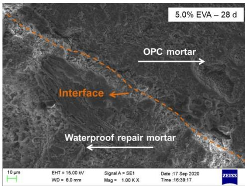
**Figure 7.** Interfacial transition zone between EVA powder modified CSA cement waterproof repairing mortar and OPC mortar
