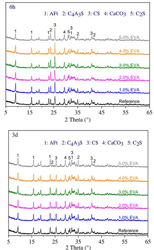
**Figure 9.** XRD patterns of CSA cement hydration samples at the hydration age of 6 h and 3 d
