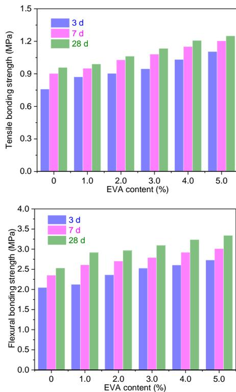
**Figure 5.** Tensile bonding strength and flexural bonding strength of EVA powder modified CSA cement waterproof repair mortar
