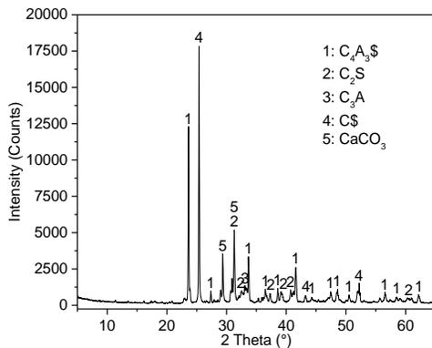
Figure 1. XRD pattern of CSA cement
