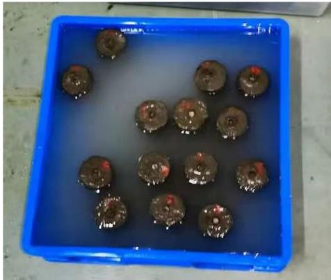
Figure 2. Submerged curing
