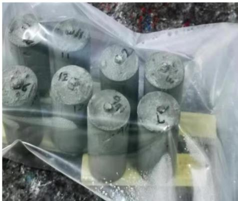
Figure 3. Sealed curing
