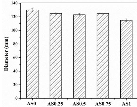
**Figure. 1** Fluidity of cement pastes with various  $\text{Al}_2(\text{SO}_4)_3$
