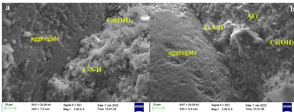
**Figure. 4** Microstructure of (a) blank cement mortar samples, (b) AS0.25 cement mortar samples.
