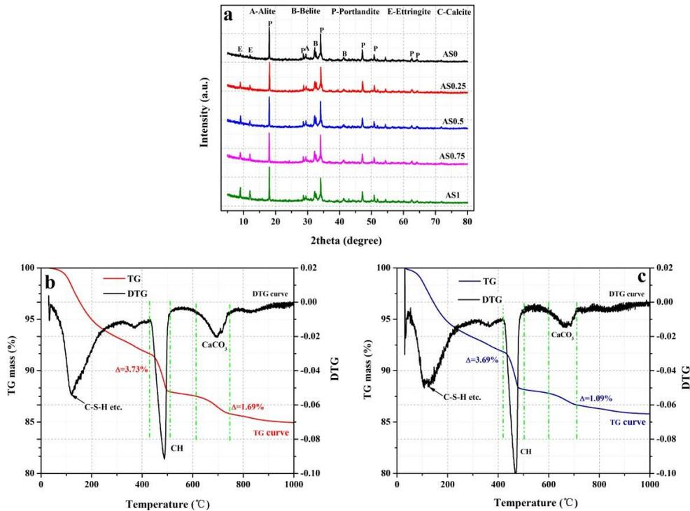
**Figure. 3** Hydration products analysis of cement pastes with various  $\text{Al}_2(\text{SO}_4)_3$ : (a) XRD, (b) TG of AS0 samples, (c) TG of AS0.25 cement paste samples.
