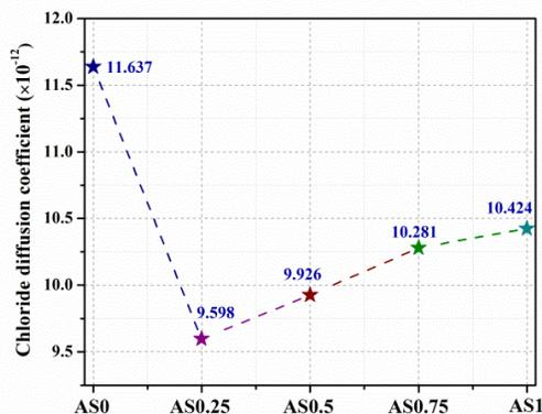
Figure. 6 Chloride ion migration coefficient of cement mortars with various  $Al_2(SO_4)_3$ .
