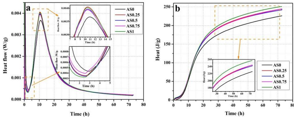
**Figure. 2** Heat of hydration of cement pastes with various  $\text{Al}_2(\text{SO}_4)_3$ : (a) heat flow, (b) heat.
