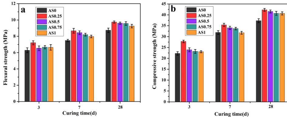
Figure. 5 Mechanical properties of cement mortars with various  $Al_2(SO_4)_3$ : (a) flexural strength, (b) compressive strength.
