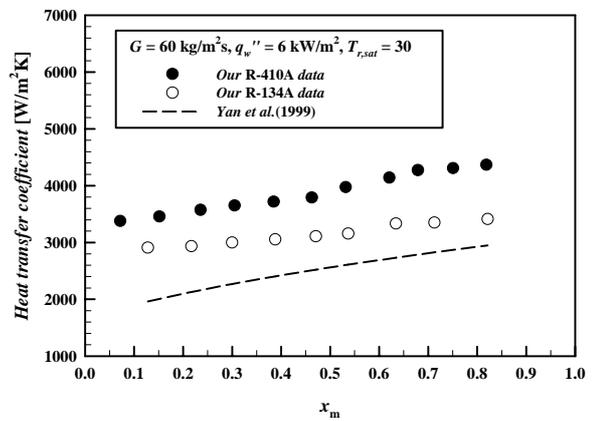
Figure 7 : Comparison of the present heat transfer data with those for plate heat exchanger from Yan et al. and our R-134A data
