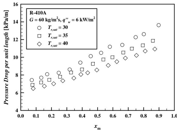
Figure 10 : Frictional pressure drop variations with the mean vapor quality for various saturation temperatures at  $G = 60 \text{ kg/m}^2\text{s}$  and  $q_w'' = 6.0 \text{ kW/m}^2$
