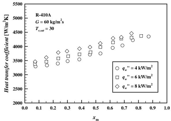
Figure 5 : Variations of condensation heat transfer coefficient with mean vapor quality for various heat fluxes at  $G = 60 \text{ kg/m}^2\text{s}$  and  $T_{r,sat} = 30$
