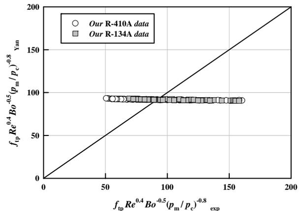
Figure 11 : Comparison of the present pressure drop data with those for plate heat exchanger from Yan et al.
