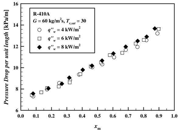
Figure 9 : Frictional pressure drop variation with the mean vapor quality for various heat fluxes at  $G = 60 \text{ kg/m}^2\text{s}$  and  $T_{r,sat} = 30$
