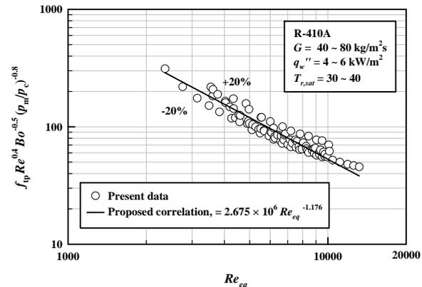
Figure 13 : Comparison of the proposed correlation for friction factor with the present data
