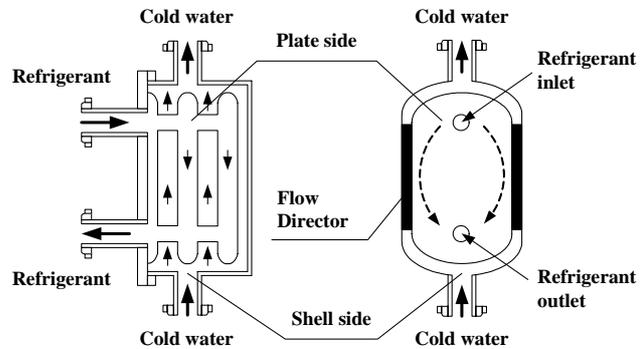
Figure 3 : Details of condensation flow direction
