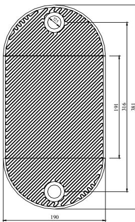
Figure 2 : Schematic diagram of heat transfer plate
