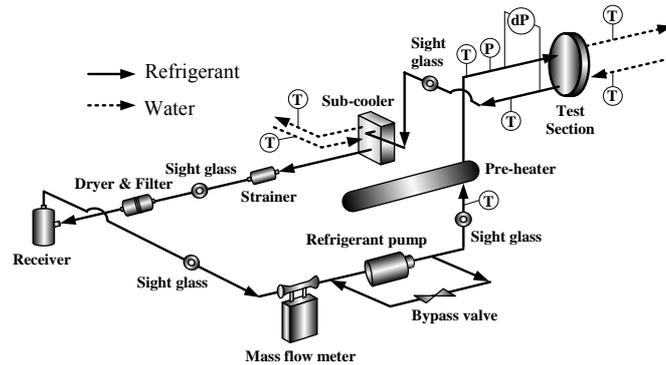
Figure 1 : Schematic diagram of Oblong Shell and Plate heat exchanger
