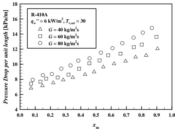
Figure 8 : Frictional pressure drop variation with the mean vapor quality for various mass fluxes at  $q_w'' = 6.0 \text{ kW/m}^2$  and  $T_{r,sat} = 30$
