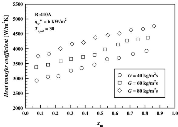
Figure 4 : Variations of condensation heat transfer coefficient with mean vapor quality for various mass fluxes at  $q_w'' = 6.0 \text{ kW/m}^2$  and  $T_{r,sat} = 30$
