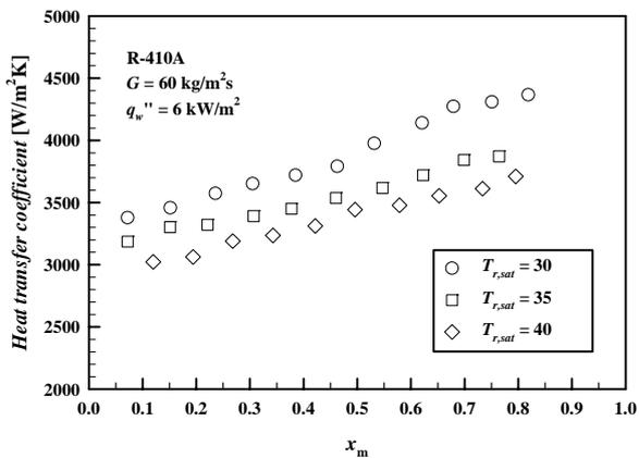
Figure 6 : Variations of condensation heat transfer coefficient with mean vapor quality for various saturation temperatures at  $G = 60 \text{ kg/m}^2\text{s}$  and  $q_w'' = 6.0 \text{ kW/m}^2$
