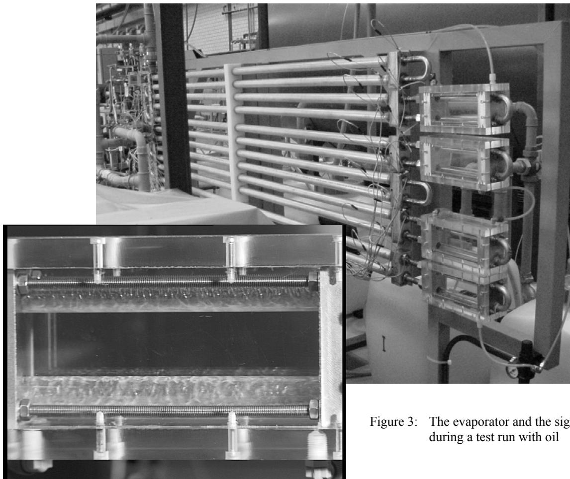
Figure 3: The evaporator and the sight glass during a test run with oil
