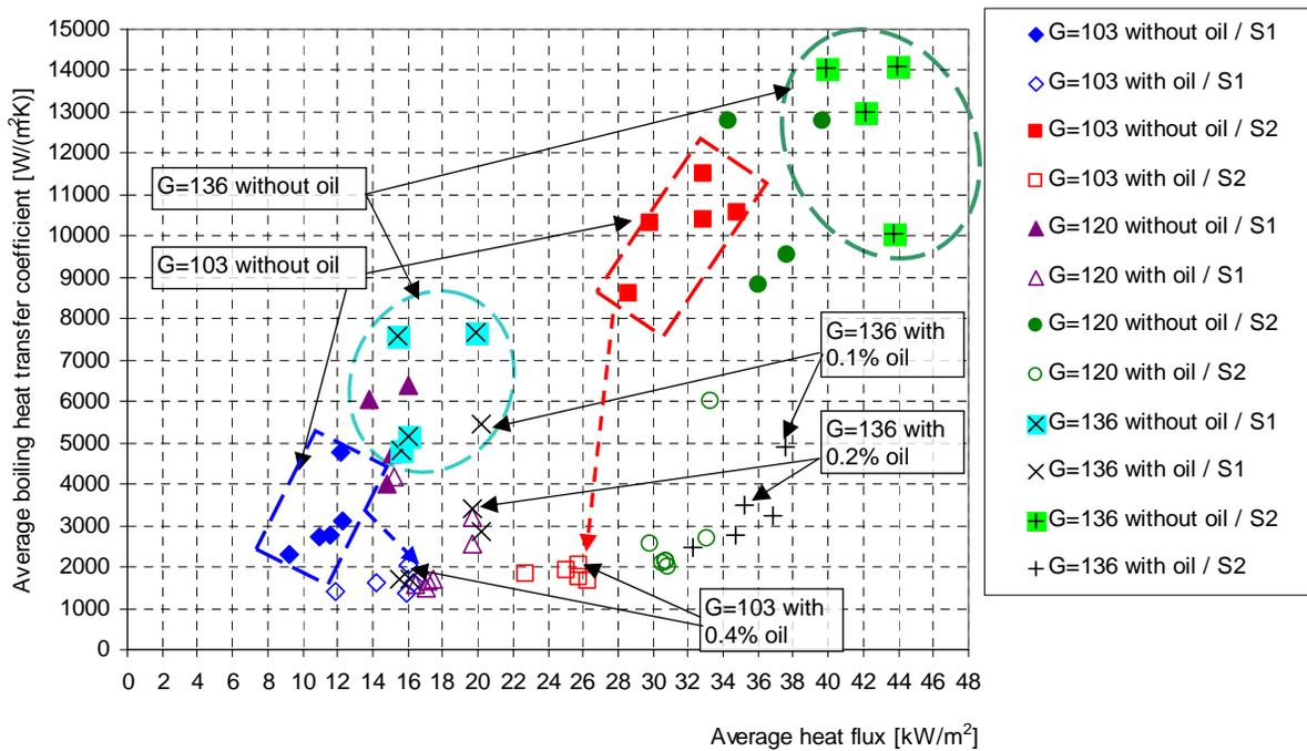
Figure 7: Average values of the heat transfer coefficient for flow boiling of ammonia in the sectors S1 and S2 {for selected mass velocities  $G$  [kg/(m<sup>2</sup>s)]} versus average heat flux in the corresponding sector of the evaporator
