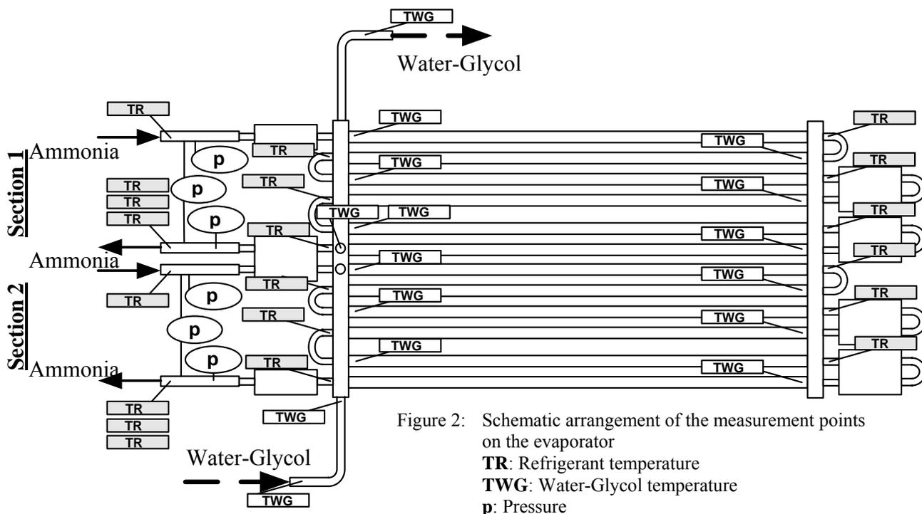
Figure 2: Schematic arrangement of the measurement points on the evaporator
