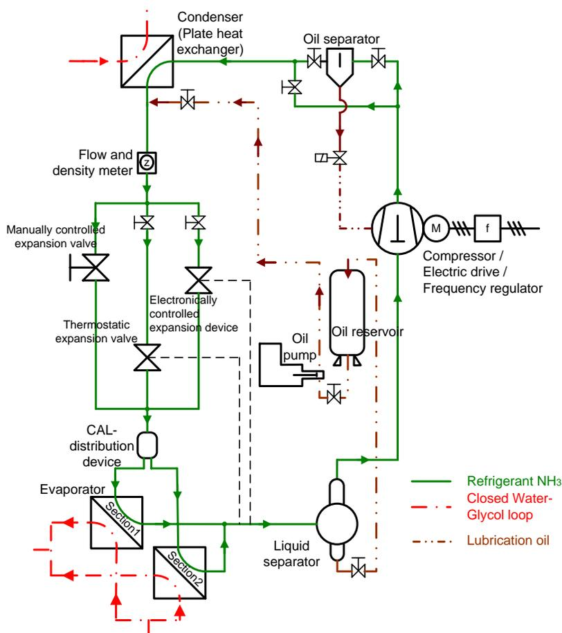
Figure 1: Flow circuit diagram of the test facility
