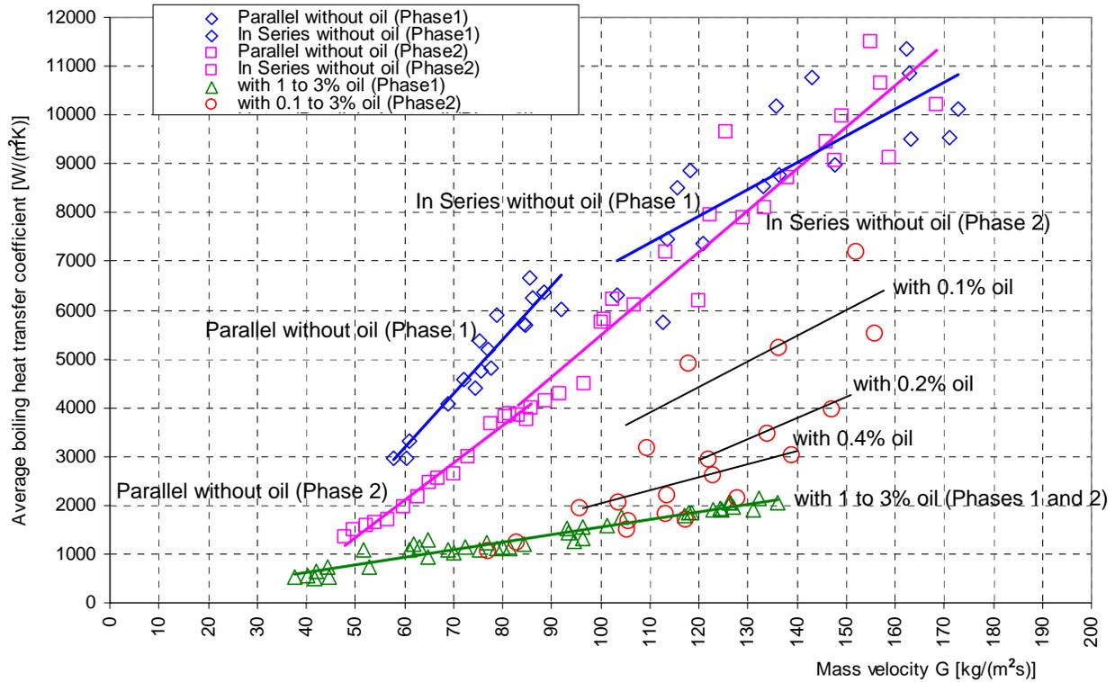
Figure 6: Average values of the heat transfer coefficient  $h_{NH_3}$  for flow boiling of ammonia versus mass velocity for different oil contents in ammonia
