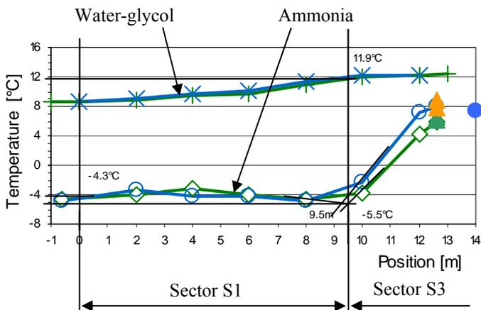
Figure 4: Temperature profiles along the evaporator coils during test runs with evaporator sections operated in parallel (Evaporation from  $x_{\text{evap\_in}} = 0.15$  to 1.0 in Sector S1, Overheating in Sector S3)
