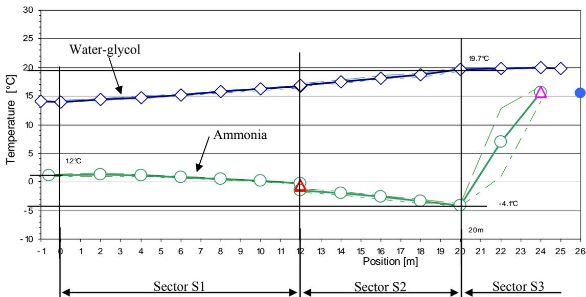
Figure 5: Temperature profiles along the evaporator coils during test runs with evaporator sections operated in series (Evaporation from  $x_{\text{evap\_in}} = 0.15$  to 1.0 in Sectors S1 and S2, Overheating in Sector S3)
