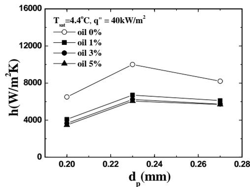
Fig. 13 Effect of pore diameter on the heat transfer coefficients of R-123/oil mixtures at  $T_{\text{sat}} = 4.4\text{C}$ ,  $q'' = 40 \text{ kW/m}^2$
