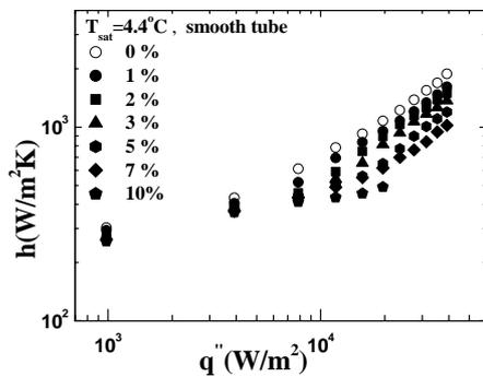
Fig. 5 Effect of oil on boiling heat transfer coefficients of the smooth tube at  $T_{\text{sat}} = 4.4^\circ\text{C}$
