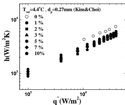
Fig. 7 Effect of oil on heat transfer coefficients of  $d_p = 0.27$  mm tube ( $T_{\text{sat}} = 4.4^\circ\text{C}$ )
