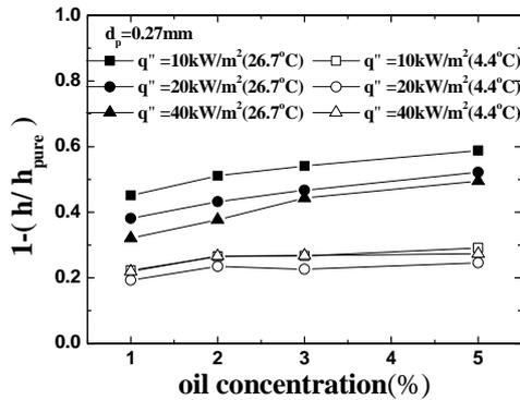
Fig. 9 Effect of oil on the heat transfer degradation for  $d_p = 0.27\text{mm}$  tube
