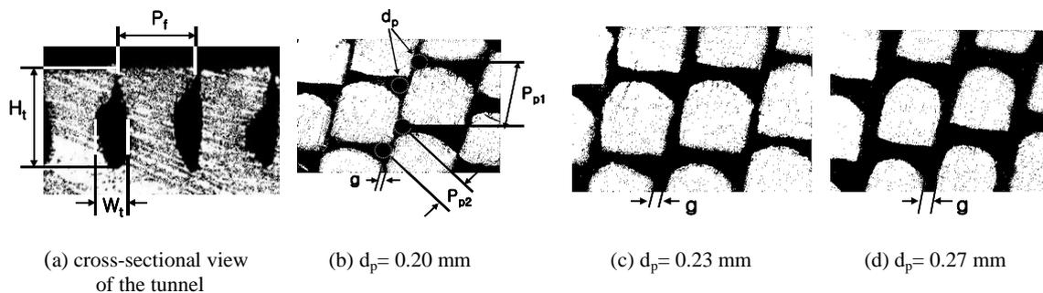
Fig. 2 Enlarged photos showing the present enhanced geometry: (a) cross-sectional view of the tunnel, (b) tube with  $d_p = 0.20$  mm, (c) tube with  $d_p = 0.23$  mm, (d) tube with  $d_p = 0.27$  mm
