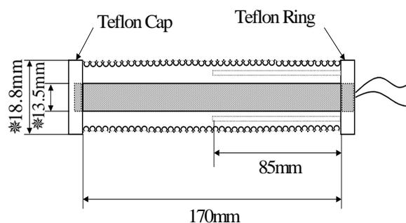
Fig. 4 Detailed sketch of the test tube.
