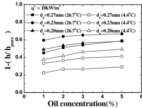
Fig. 12 Effect of oil on heat transfer degradation at  $q'' = 10\text{ kW/m}^2$
