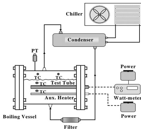
Fig. 3 Schematic drawing of the experimental apparatus.
