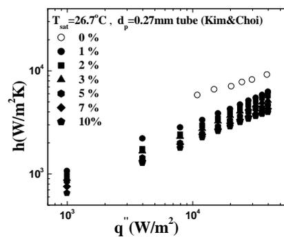
Fig. 8 Effect of oil on heat transfer coefficients of  $d_p = 0.27$  mm tube ( $T_{\text{sat}} = 26.7^\circ\text{C}$ )
