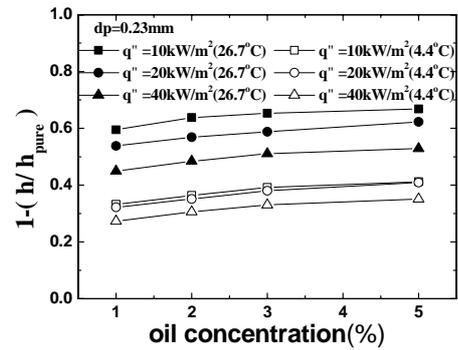
Fig. 10 Effect of oil on the heat transfer degradation for  $d_p = 0.23\text{mm}$  tube
