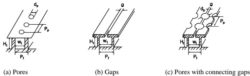
Fig. 1 Characteristic dimensions of structured enhanced tubes
