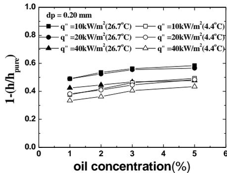
Fig. 11 Effect of oil on the heat transfer coefficients for  $d_p = 0.20\text{ mm}$  tube
